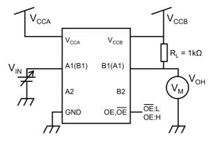
Fig. 14.1 Test Circuit
