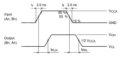
Fig. 13.3 AC Waveform of tPLH, tPHL
