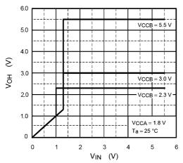
Fig. 14.2 Input/Output Characteristics (Typ.)  $V_{CCA} = 1.8 V$ , T<sub>a</sub> = 25 °C
