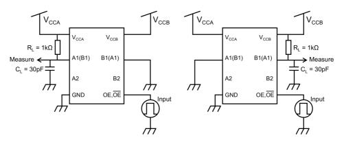
Fig. 13.2 t<sub>PLZ</sub>, t<sub>PZL</sub> Test Circuits
