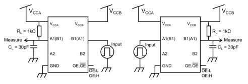
Fig. 13.1 t<sub>PLH</sub>, t<sub>PHL</sub> Test Circuits
