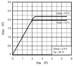
Fig. 15.3 Input/Output Characteristics (Typ.)  $V_{CCA}$  = 2.3 V, T<sub>a</sub> = 25 °C
