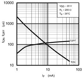
Fig. 12.1.7  $t_{ON}$ ,  $t_{OFF}$  -  $I_F$
