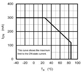
Fig. 12.1.2 I<sub>ON</sub> - T<sub>a</sub>
