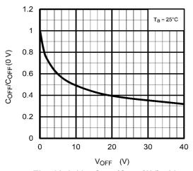
Fig. 12.1.11 C<sub>OFF</sub>/C<sub>OFF</sub>(0V) - V<sub>OFF</sub>
