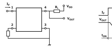
Fig. 11.1 Switching Time Test Circuit and Waveform
