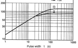
The test curves of the package surface temperature,  $T_C$  [°C], and the junction temperature,  $T_j$  [°C], when Ta = 25°C and current flows between the OUT1 and OUT2 outputs on a PCB are shown below:
