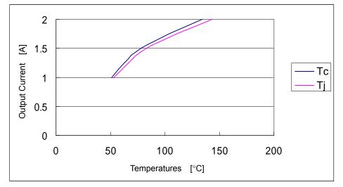
Conditions: Ta = 25°C VM = 24 V IN2, PWM,  $V_{RFE}$  = 5 V RSGND = GND TISD; 20 k  $\Omega$ , OSC = GND IN1 = -100  $\mu$ A (Diode voltage monitor circuit), on a PCB
