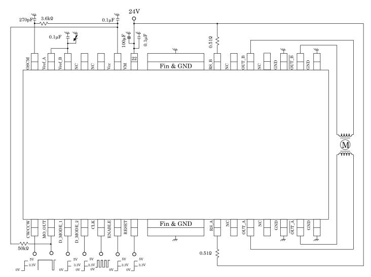
Note: Bypass capacitors should be added as necessary.
