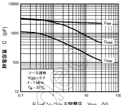
図 8.8 静電容量 -  $V_{DS}$
