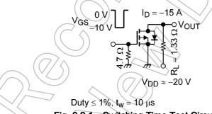
Fig. 6.2.1 Switching Time Test Circuit
