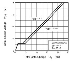
Fig. 7.11 Dynamic Input Characteristics
