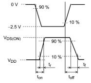
Fig. 5.3.1 Test Circuit of Switching Time
