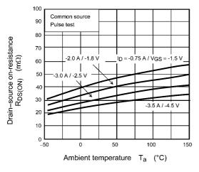
Fig. 7.5 R<sub>DS(ON)</sub> - T<sub>a</sub>
