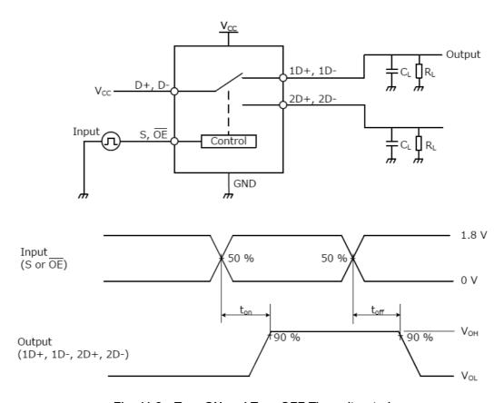
Fig. 11.2 Turn-ON and Turn-OFF Times (ton, toff)
