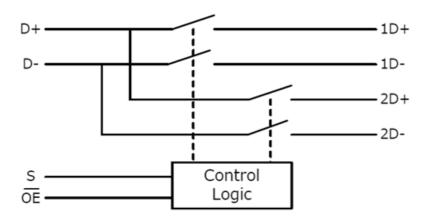
Fig. 6.1 Block Diagram
