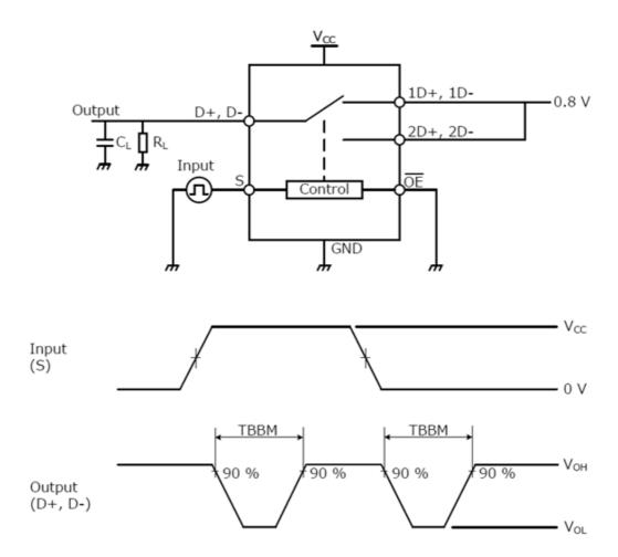
Fig. 11.3 Break Before Make (TBBM)
