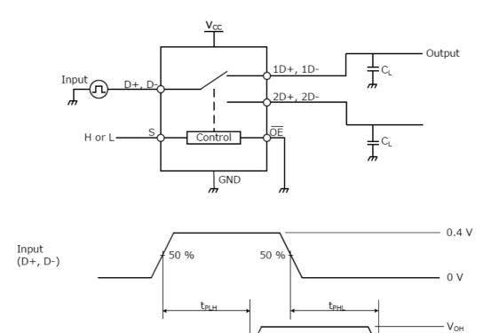
Fig. 11.1 Propagation Delay Time (t<sub>PLH</sub>, t<sub>PHL</sub>)
