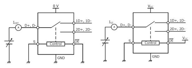
Fig. 11.10 Power-OFF Leakage Current
