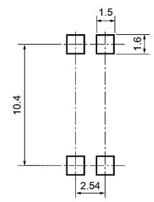
Fig. 18.2 Lead forming and taping option (LF4), (TP4)
