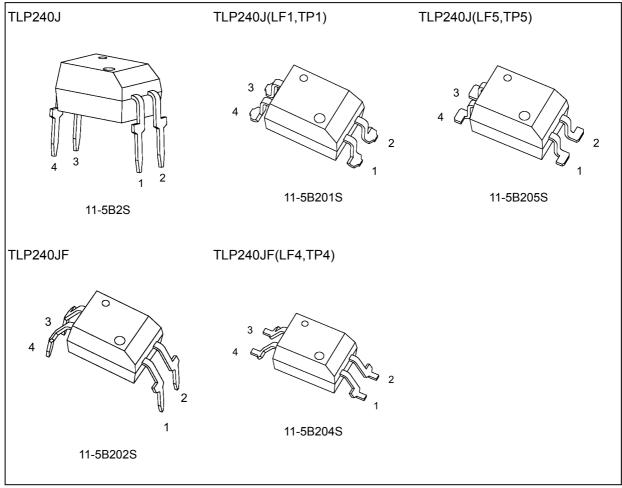
Note: Through-hole type: TLP240J, TLP240JF Lead forming option: (LF1), (LF4), (LF5) Taping option: (TP1), (TP4), (TP5)
