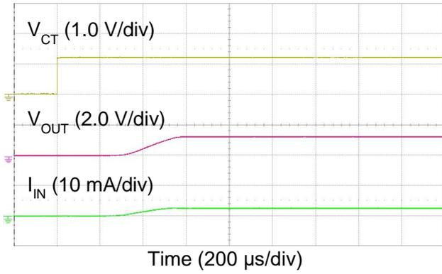
$V_{IN} = 1.2\text{ V}$ ,  $C_L = 4.7\ \mu\text{F}$ ,  $R_L = 500\ \Omega$
