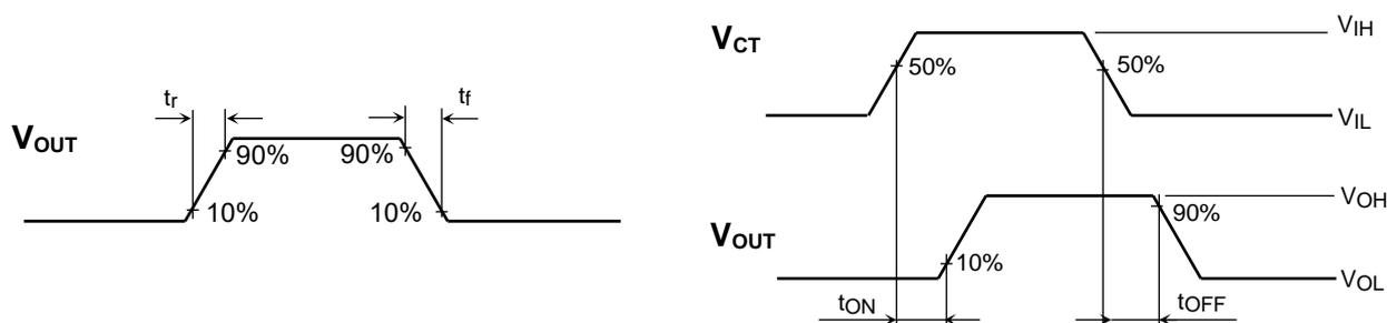
Figure 1 t<sub>r</sub>, t<sub>f</sub>, t<sub>ON</sub>, t<sub>OFF</sub> Waveforms
