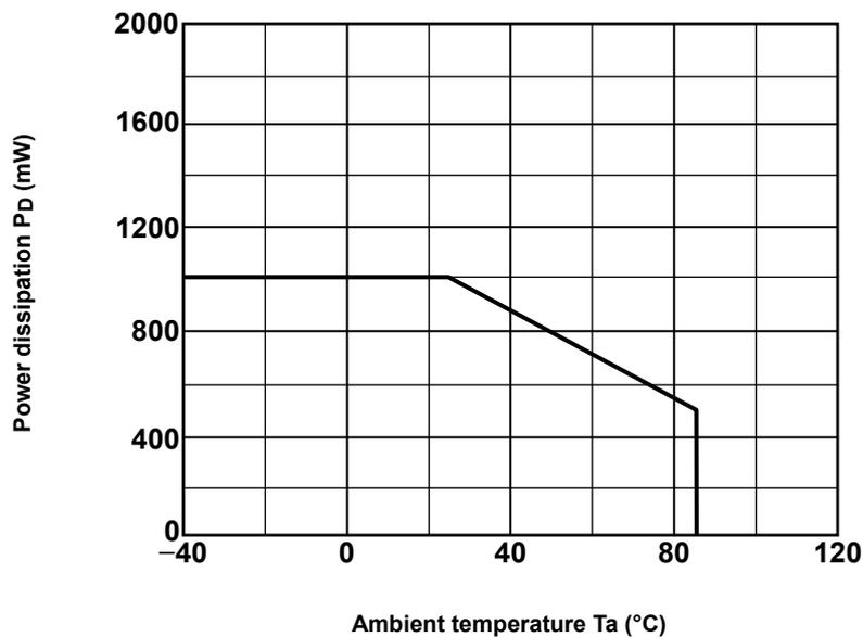
Please allow sufficient margin when designing a board pattern to fit the expected power dissipation. Also take into consideration the ambient temperature, input voltage, output current etc. and applying the appropriate derating for allowable power dissipation during operation.
