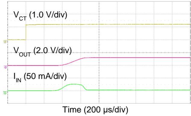
$V_{IN} = 1.8\text{ V}$ ,  $C_L = 0.1\ \mu\text{F}$ ,  $R_L = 500\ \Omega$
