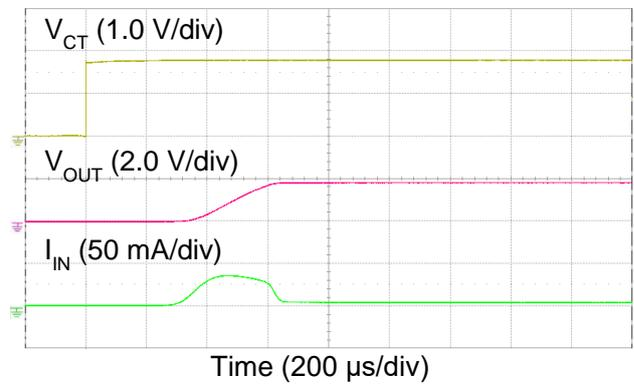
$V_{IN} = 3.3\text{ V}$ ,  $C_L = 0.1\ \mu\text{F}$ ,  $R_L = 500\ \Omega$
