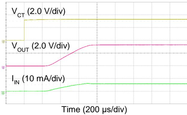
$V_{IN} = 3.3\text{ V}$ ,  $C_L = 4.7\ \mu\text{F}$ ,  $R_L = 500\ \Omega$
