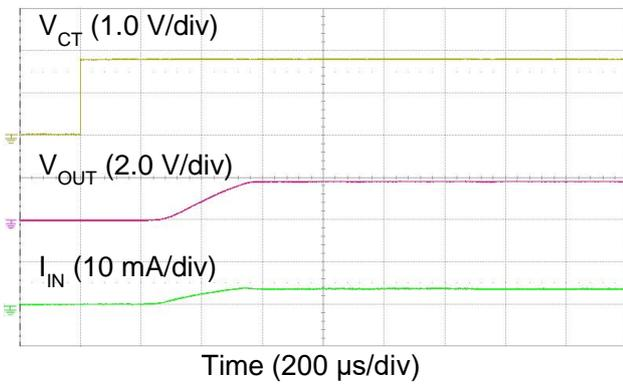
$V_{IN} = 1.8\text{ V}$ ,  $C_L = 4.7\ \mu\text{F}$ ,  $R_L = 500\ \Omega$
