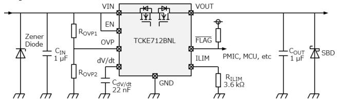
NOTE: Select Zener diodes and SBDs considering the maximum rating of eFuse IC.
