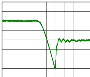
Figure 2.8 Example of a waveform of a super-fast-recovery diode (S-FRD) during t_{rr}
