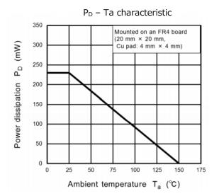
Figure 5.3 USC Power Dissipation P<sub>D</sub> – Ta characteristic example
