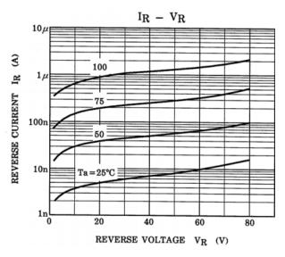
Figure 4.4 I<sub>R</sub>-V<sub>R</sub> Temperature Characteristics
