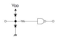
(g) Delay time control circuit
