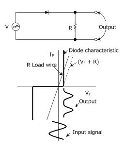
Figure 4.5 Diode Detection Operation
