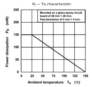
Figure 5.1 ESC Power Dissipation P<sub>D</sub> – Ta characteristic example
