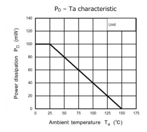
Figure 5.5 S-Mini Power Dissipation PD – Ta characteristic example-
