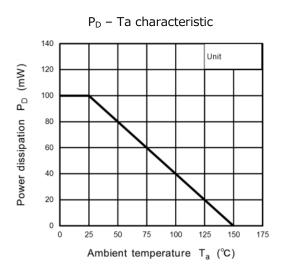
Figure 5.4 USM Power Dissipation P<sub>D</sub> – Ta characteristic example
