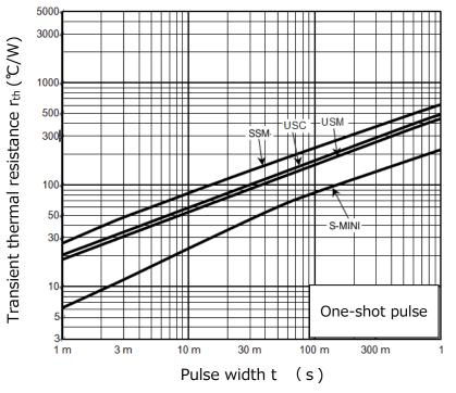
Figure 6.1 r<sub>th</sub> by Diode Package-t
