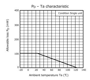
Figure 5.2 SSM Power Dissipation PD – Ta characteristic example
