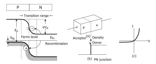
Figure 4.1 Energy Level Diagram of PN Junctions
