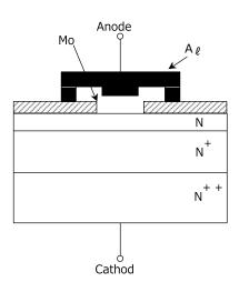
Figure 4.7 Structural Diagram of Shotky Barrier Diode
