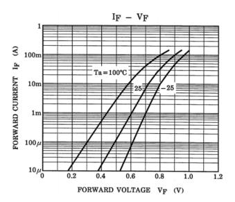
Figure 4.3 IF-VF Temperature Characteristics
