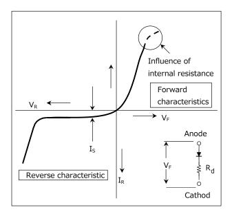
Figure 4.2 Static Characteristics of Diodes
