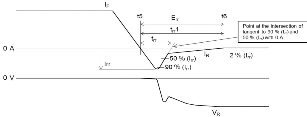
$$E_{rr} = \int_{t_5}^{t_6} (I_R \times V_R) dt$$
