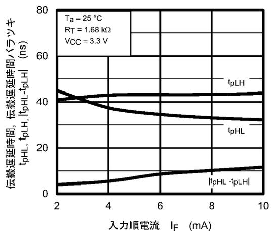
図 12.2.12  $t_{pHL}, t_{pLH}, |t_{pHL} - t_{pLH}| - I_F$
