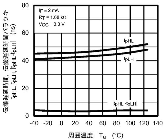
図 12.2.10  $t_{pHL}, t_{pLH}, |t_{pHL} - t_{pLH}| - T_a$
