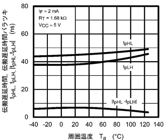
図 12.2.11  $t_{pHL}, t_{pLH}, |t_{pHL} - t_{pLH}| - T_a$
