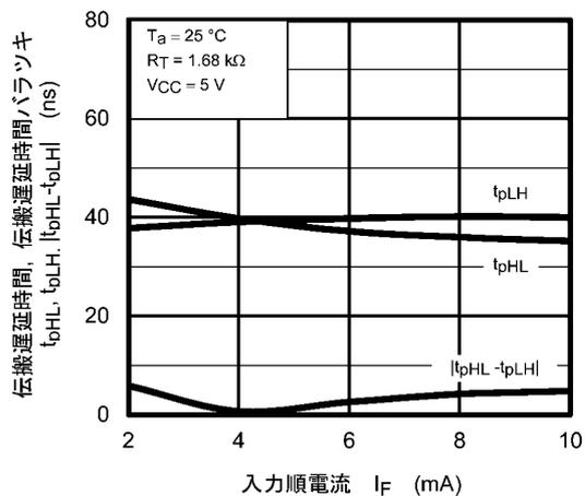
図 12.2.13  $t_{pHL}, t_{pLH}, |t_{pHL} - t_{pLH}| - I_F$
