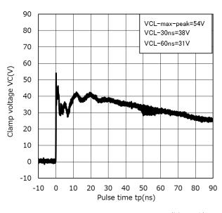
Clamp Waveform +8 kV (Note 3)
