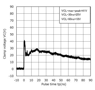
Clamp Waveform +8 kV (Note 3)
