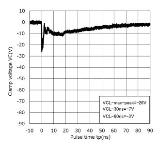
Clamp Waveform -8 kV (Note 3)
