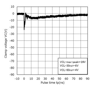
Clamp Waveform -8 kV (Note 3)
