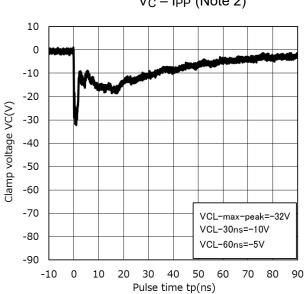
Clamp Waveform +8 kV (Note 3)
