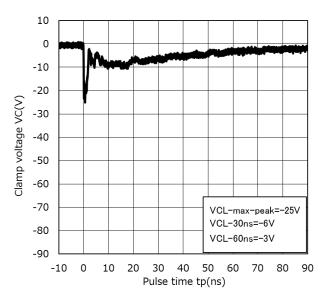
Clamp Waveform -8 kV (Note 3)
