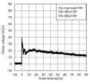
Clamp Waveform +8 kV (Note 3)
