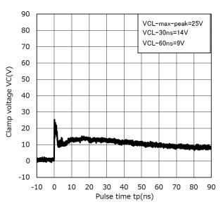
Clamp Waveform +8 kV (Note 3)
