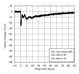
Clamp Waveform -8 kV (Note 3)
