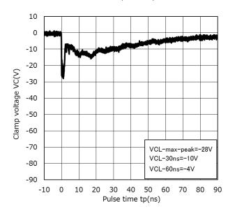
Clamp Waveform -8 kV (Note 3)
