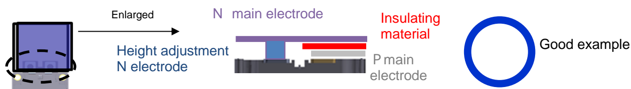
Figure 2.5.5 An example of recommended parallel electrodes and insulation for P and N main electrodes
