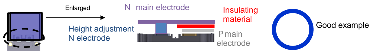
Figure 2.5.5 An example of recommended parallel electrodes and insulation for P and N main electrodes
