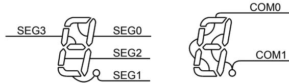
Figure 17-7 Example of COM and SEG Pin Connections
