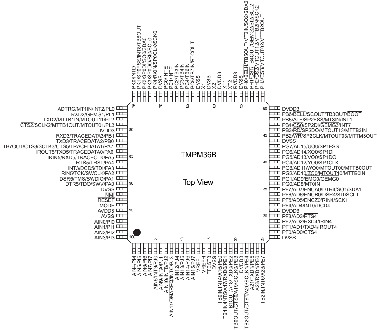
Figure 1-2 Pin Layout (LQFP100)
