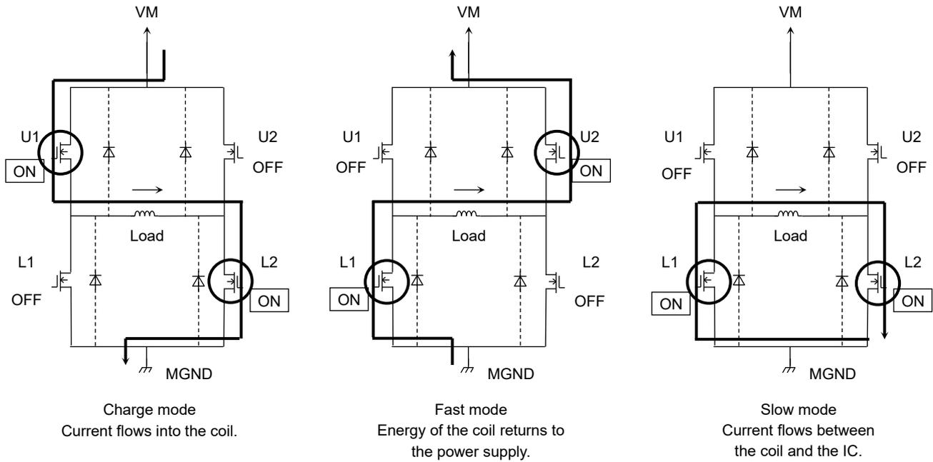
**Figure 7.23 Output Transistor Function mode**
