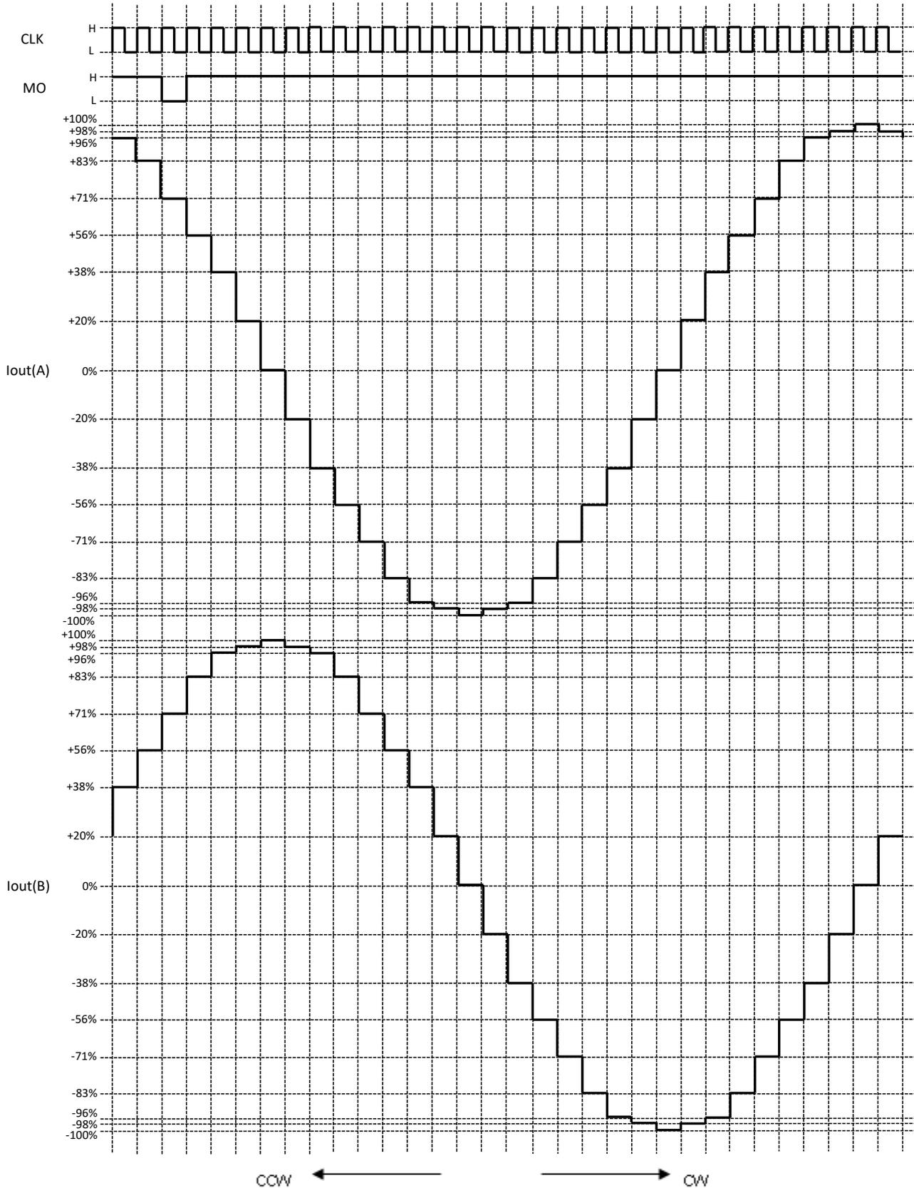
Figure 7.5 1/8 step resolution setting
