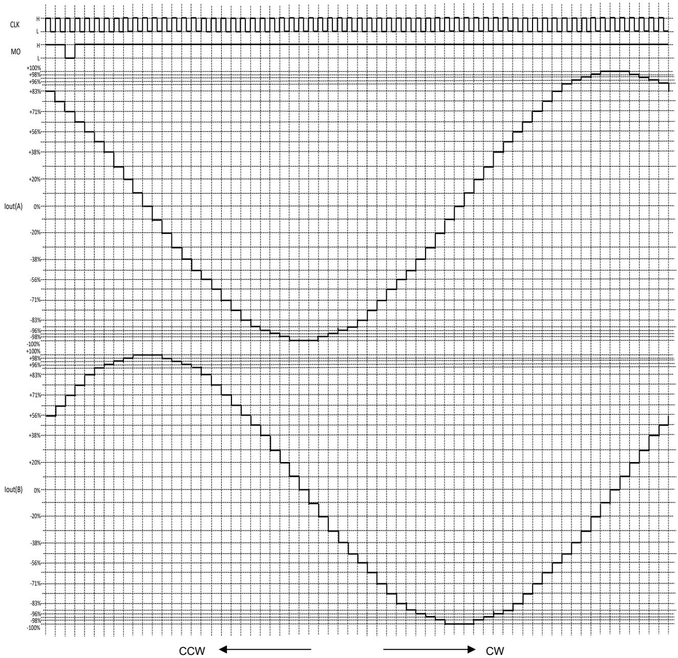
**Figure 7.6 1/16 step resolution setting**
