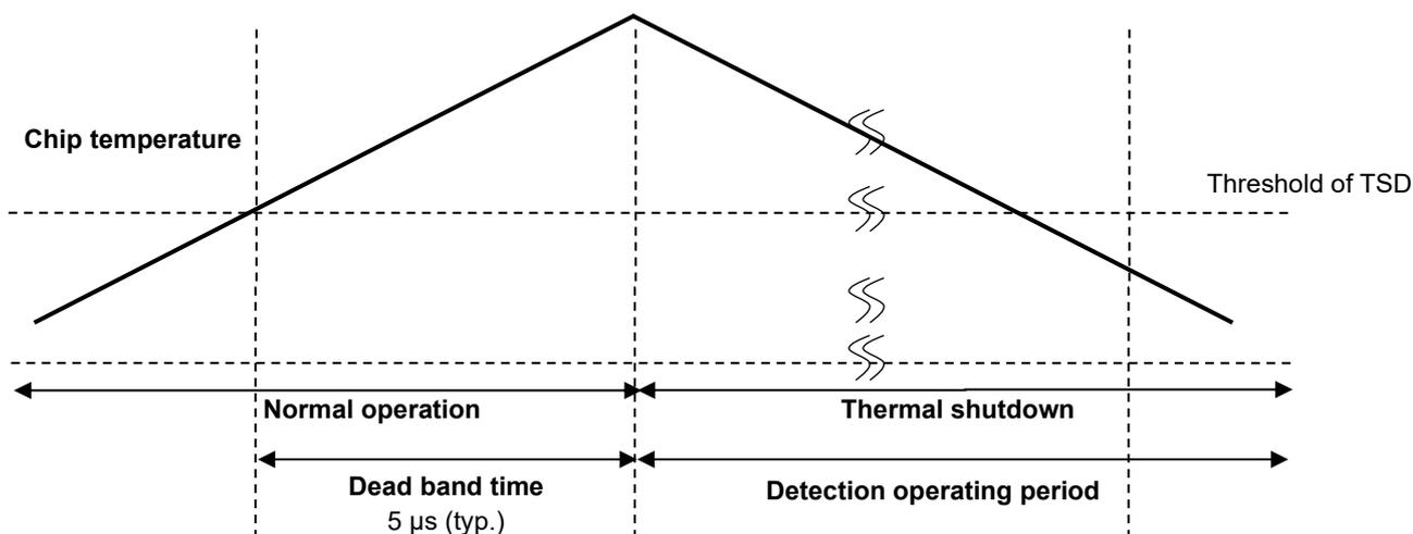
**Figure 7.25** Thermal shutdown detection
