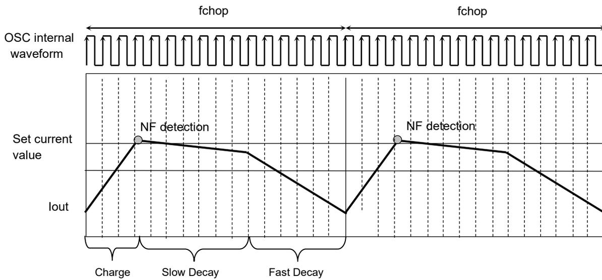
**Figure 7.9 Mixed Decay Waveform**
