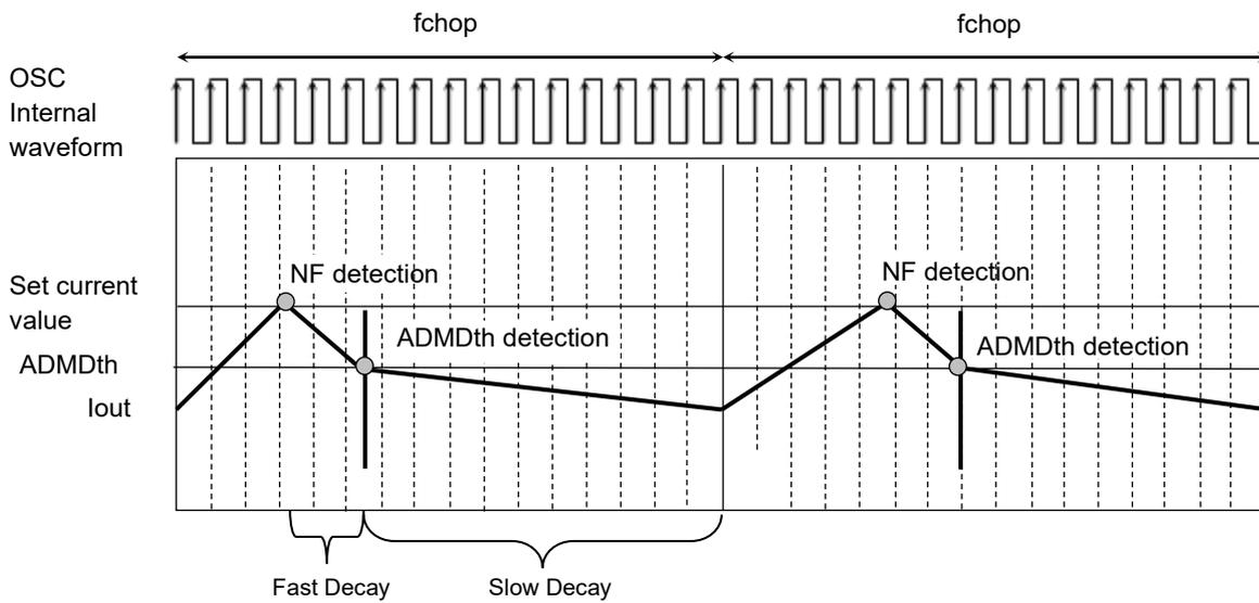
**Figure 7.17 Auto Decay Mode Current Waveform**
