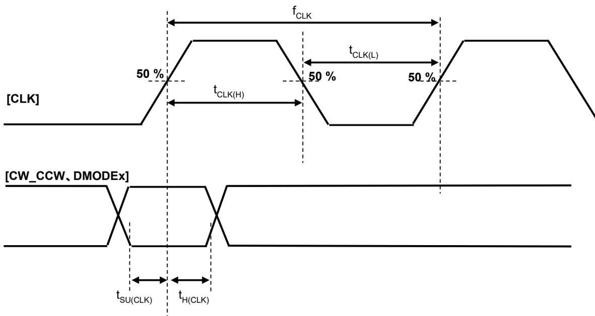
**Figure 10.2 TB67S539SFTG(Relationship between CLK and other control signals)**
