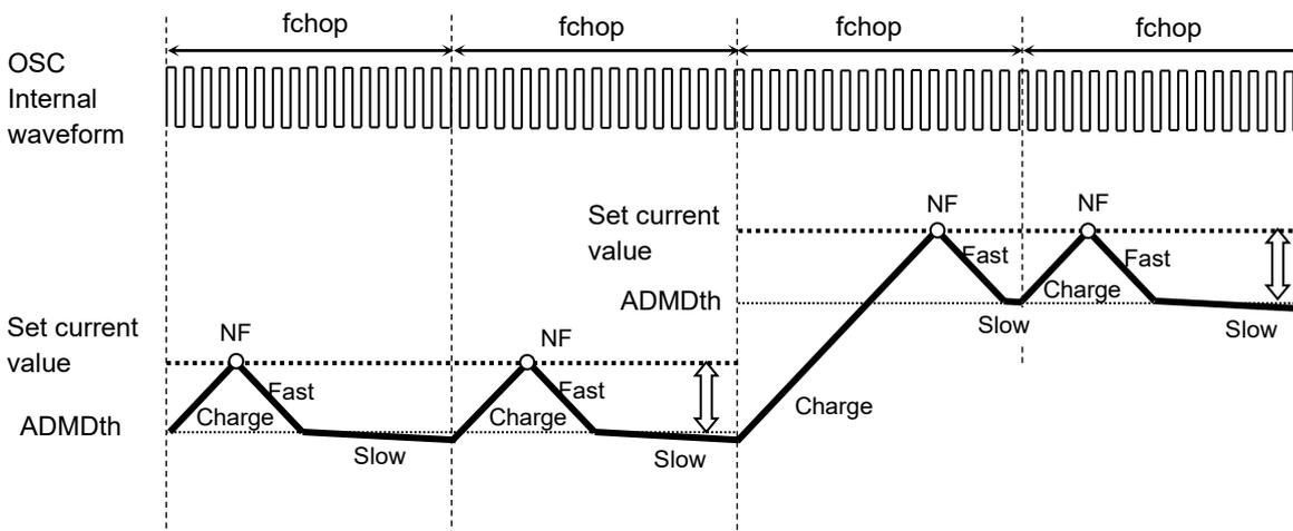
**Figure 7.18 When the next current value is increased**
