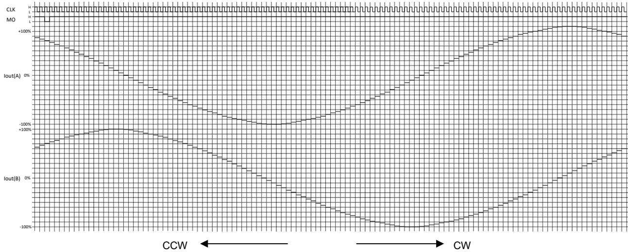
**Figure 7.7 1/32 step resolution setting**
