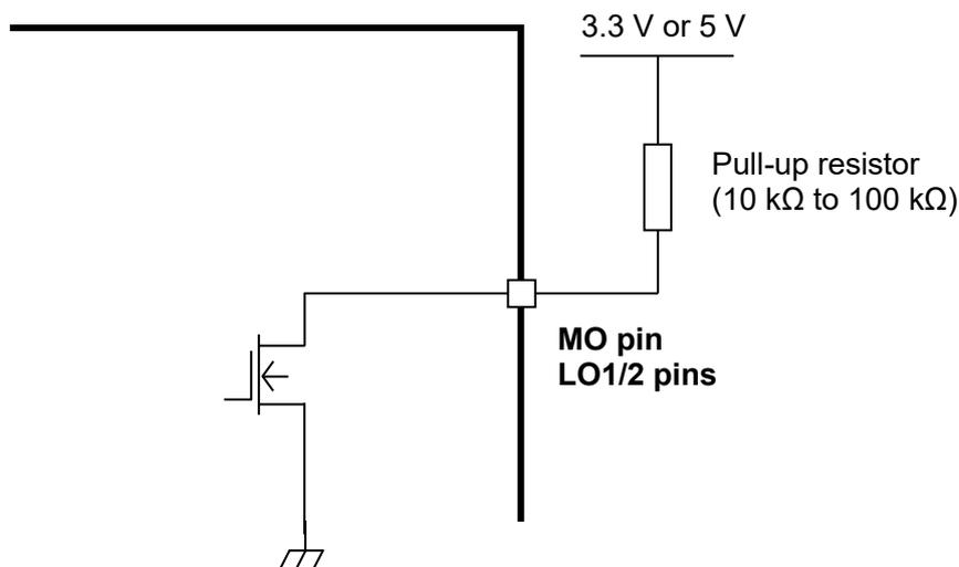
**Figure 7.22 LO function Equivalent Circuit**
