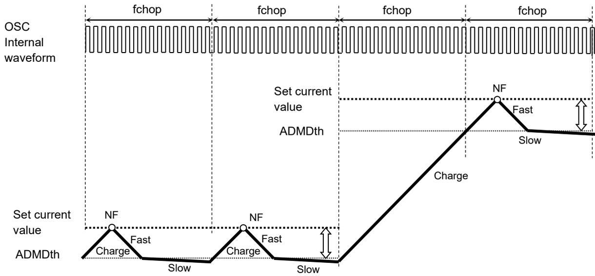
**Figure 7.19 When Charge period  $\geq 1 f_{CHOP}$  cycle**
