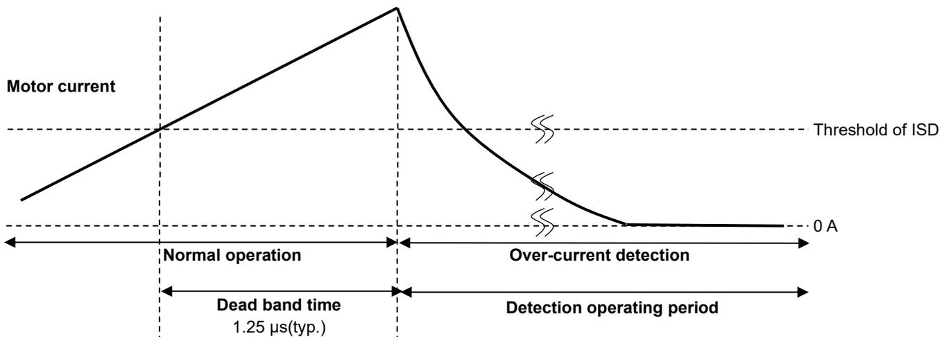
**Figure 7.27 Over-current detection timing charts**
