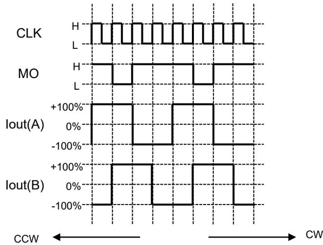
**Figure 7.1 Full step resolution setting**
