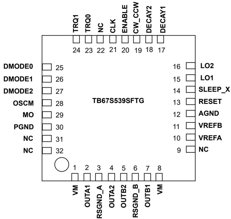
**Figure 4.1 Pin Assignments**
