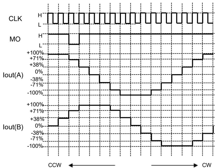
**Figure 7.4 Quarter step resolution setting**
