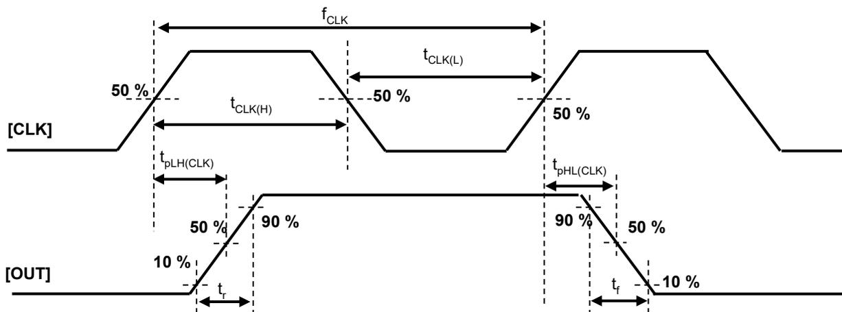
**Figure 10.1 TB67S539SFTG(Relationship between CLK and output)**
