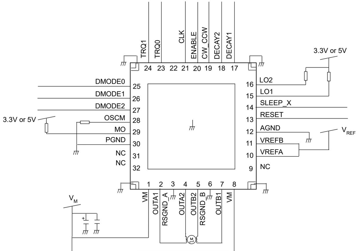
**Figure 11.1 Application Circuit Example**
