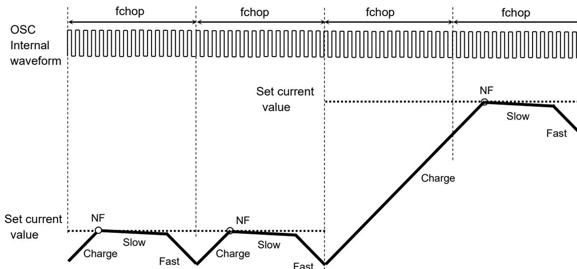
**Figure 7.13 When the Charge period is more than 1  $f_{chop}$  cycle**
