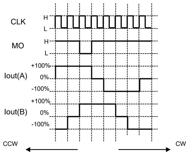
**Figure 7.2 Half step resolution (a) setting**
