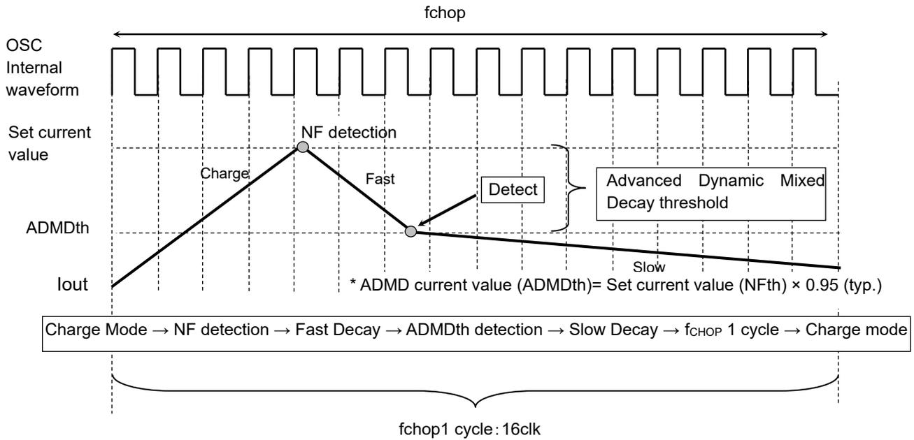
**Figure 7.15 ADMD (Advanced Dynamic Mixed Decay) Constant Current Control**
