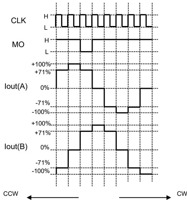
**Figure 7.3 Half step resolution (b) setting**
