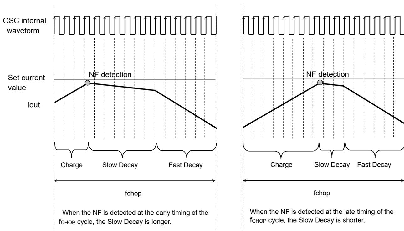
Figure 7.10 Each Time of Constant Current (1) Figure 7.11 Each Time of Constant Current (2)
