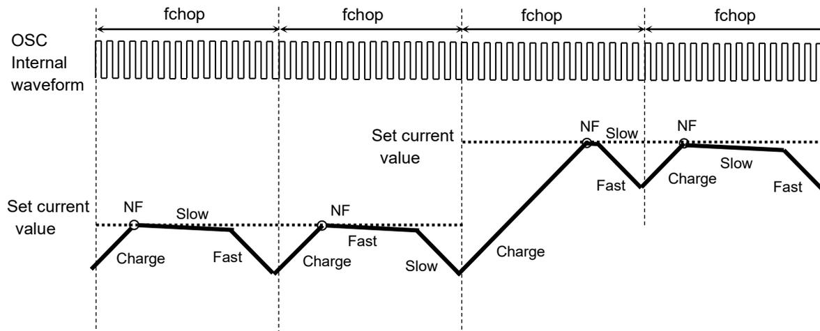
**Figure 7.12 When the set current value is increased**
