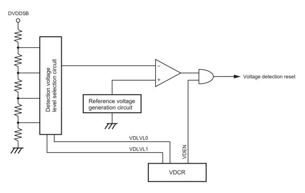
Figure 19-1 Voltage Detection Circuit)
