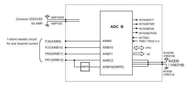
Figure 13-1 AD converters Block Diagram
