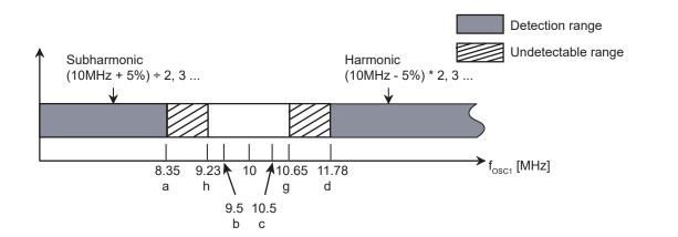
Figure 20-3 Example of detection frequency range (in case of 10MHz)
