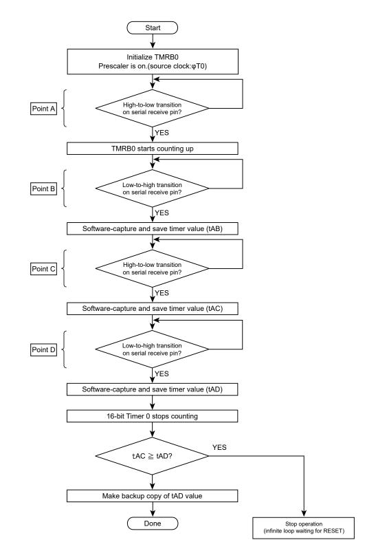
Figure 22-7 Serial operation mode receive flowchart
