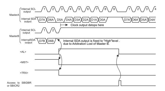
Figure 12-8 Example of Master B Lost Arbitration (D7A = D7B, D6A = D6B)
