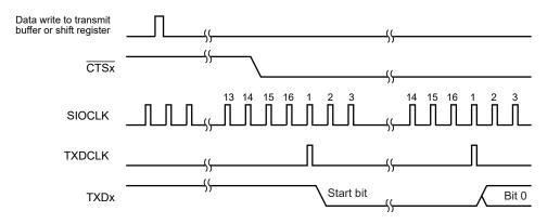
Figure 11-12 CTSx Signal timing
