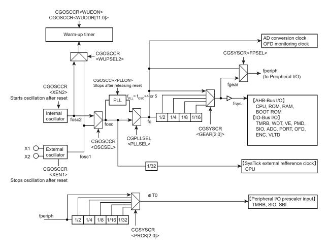
Figure 5-1 Clock Block Diagram
