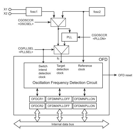
Figure 20-1 Ocsillation Frequency Detector Block diagram
