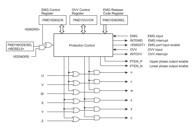
Figure 14-8 Protection Control Circuit
