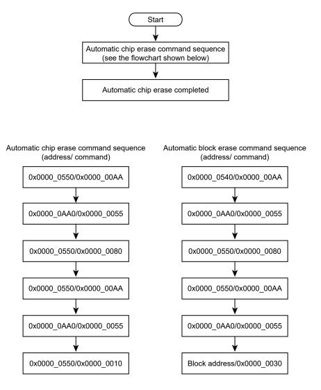
Figure 22-5 Flowchart of automatic erase
