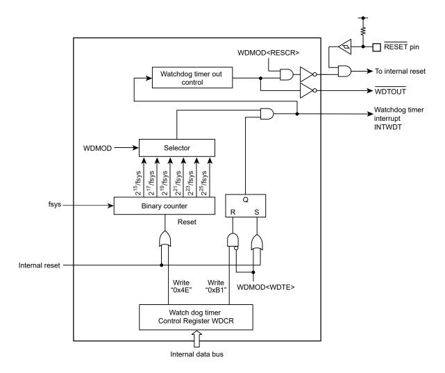
Figure 21-1 Block Diagram of the Watchdog Timer
