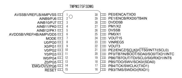
Figure 1-2 Pin Layout (SSOP30)
