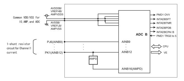
Figure 16-1 Op-Amps/Analog Converters Block Diagram
