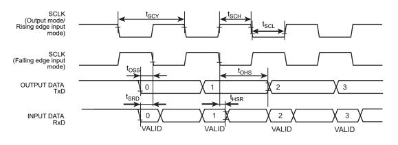
Figure 25-1 Serial channel timing(SIO)
