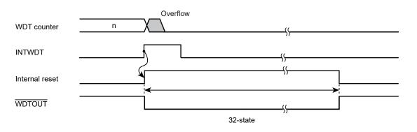
Figure 21-3 Internal reset generation
