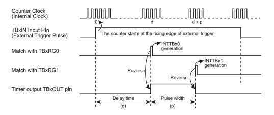
Figure 10-5 One-shot pulse generation using an external count start trigger (with a delay)
