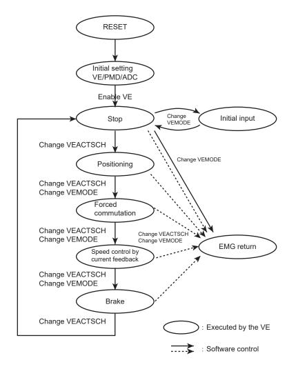
Figure 15-7 Example of Motor Control Flow
