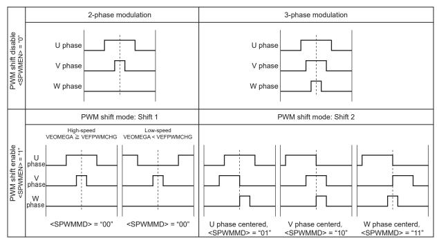
Note1) The shift-1 can be selected 2-phase modulation only. Note2) The shift-2 can be selected 3-phase modulation only. Note3) The shift-2 is necessary to set PMD registers.
