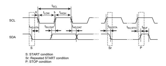
Figure 25-2 Serial Bus timing (I2C)
