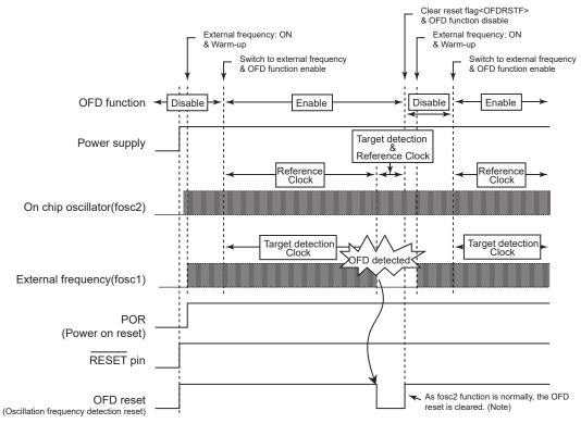
Note: The target clock is set without 10MHz into OFDMNPLLOFF and OFDMXPLLOFF. (eg, setting to 8MHz value to these registers) And when the target clock frequency is fosc1 and the reset generated by OFD, the reset might be generated continuously due to as abnormal detection until OFD detects correctly.
