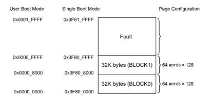
Figure 22-1 Block configuration
