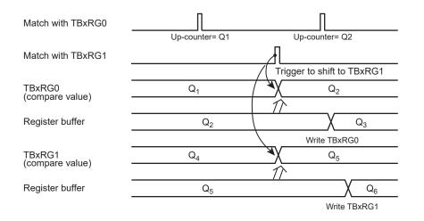
Figure 10-3 Register Buffer Operation
