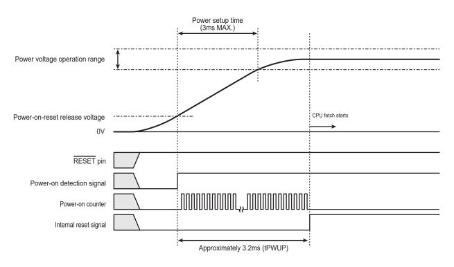
Figure 4-1 Reset Operation by Power-on Circuit
