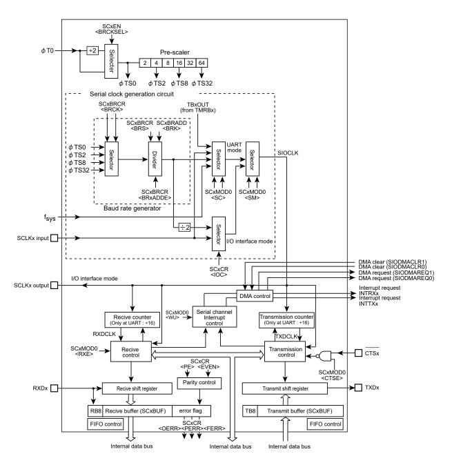
Figure 11-1 Serial Channel Block Diagram
