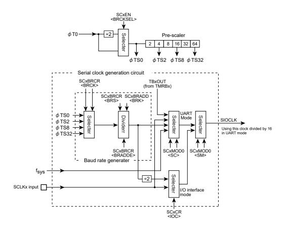
Figure 11-3 Serial clock generation circuit
