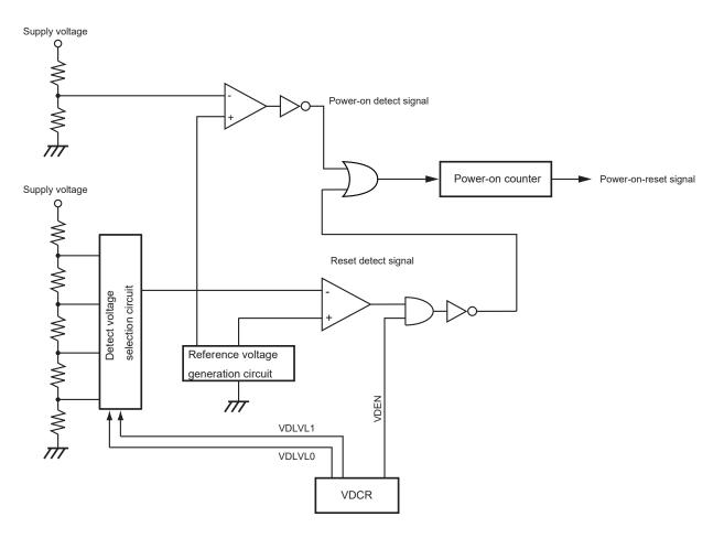
Figure 18-1 Power-on-reset circuit
