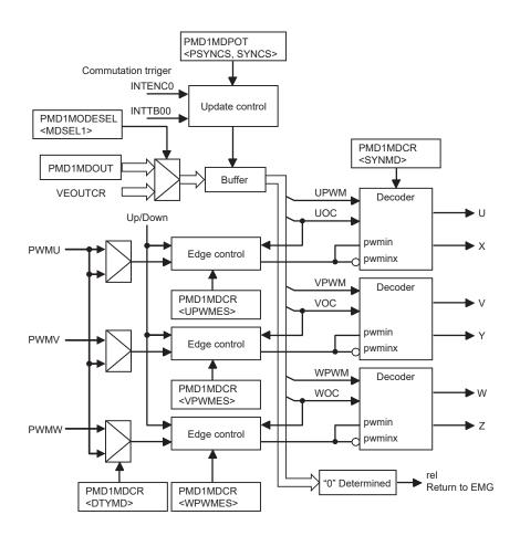
Figure 14-7 Conduction Control Circuit
