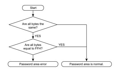
Figure 22-9 Password area check flowchart
