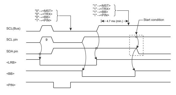
Figure 12-14 Timing Chart of Generating a Restart
