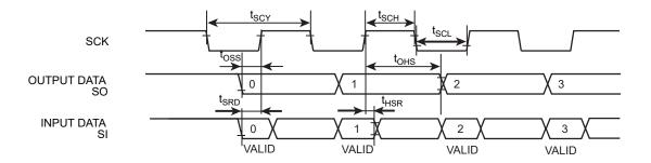
Figure 25-3 Serial Bus timing (SIO)
