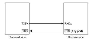
Figure 11-11 Handshake Function
