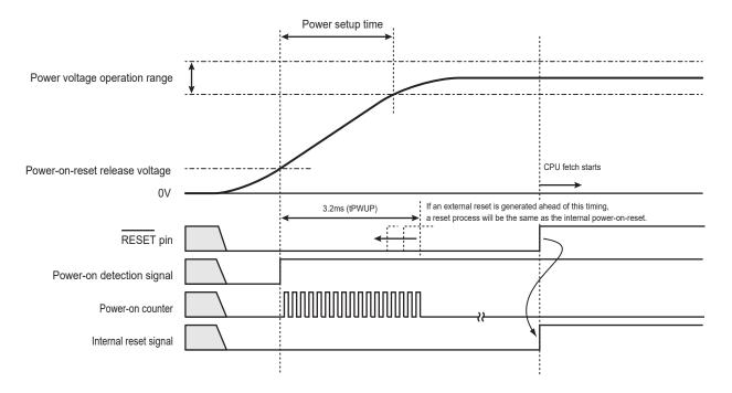
Figure 4-2 Reset Operation by RESET pin
