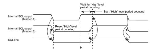
Figure 12-4 Example of Clock Synchronization
