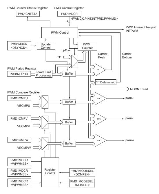
Figure 14-4 Pulse Width Modulation Circuit
