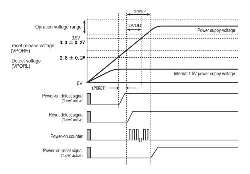
Figure 18-2 Power-on-reset operation timing
