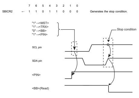
Figure 12-13 Generating the Stop Condition
