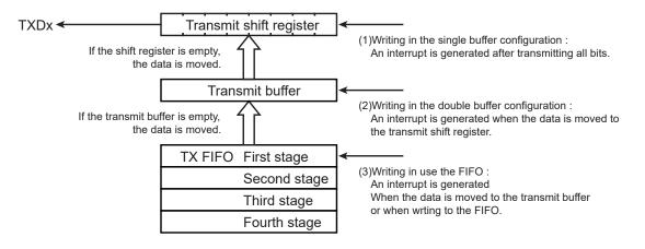
Figure 11-14 Transmit Buffer / FIFO Configuration Diagram
