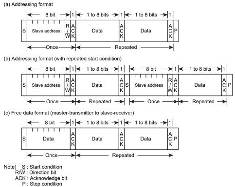
Figure 12-2 I2C Bus Mode Data Formats
