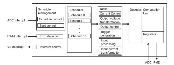
Figure 15-2 Configuration of the Vector Engine
