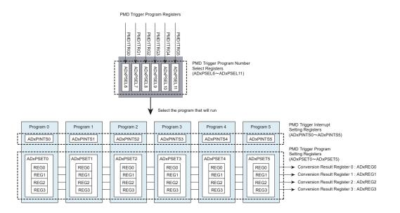
Figure 13-2 PMD Trigger Program Registers
