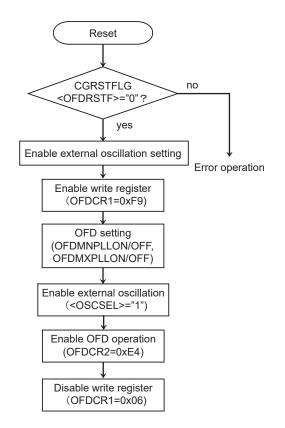
Figure 20-4 Example of operational procedure
