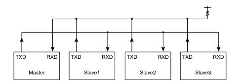
Figure 11-21 Serial Links to Use Wake-up Function
