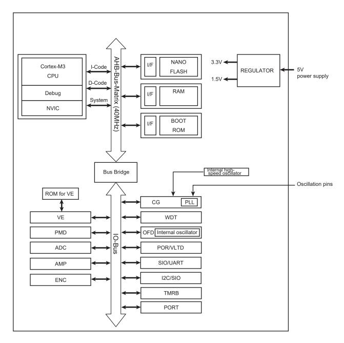
Figure 1-1 TMPM375FSDMG block diagram
