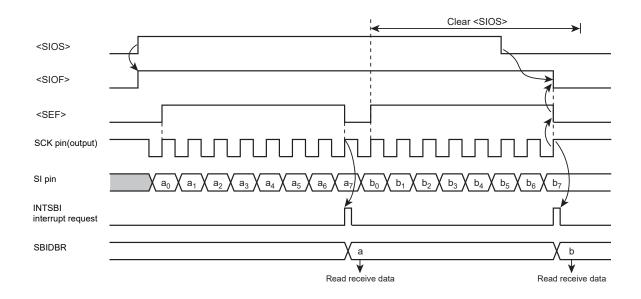
Figure 12-19 Receive Mode (Example: Internal Clock)
