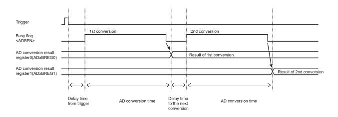
Figure 13-3 Timing chart of AD conversion
