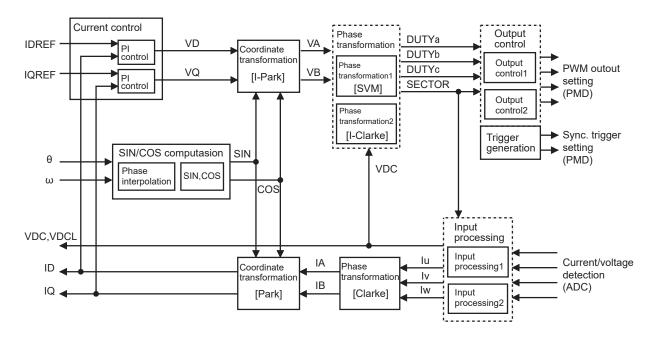
Figure 15-1 Block Diagram of Vector Control
