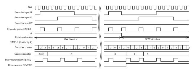
• In Sensor Timer Count mode, the Hall sensor inputs of the MCU should be connected to the U, V and W channels. The encoder counter measures the interval between two contiguous pulses of ENCLK, which is either multiplied by 4 clock (when <P3EN> = "0") derived from the decoded U and V signals or multiplied by 6 clock (when <P3EN> = "1") derived from the decoded U, V and W signals.
