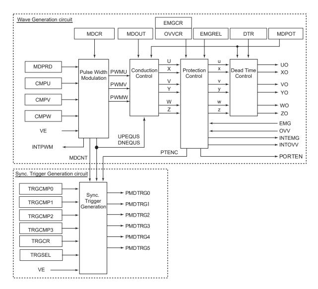
Figure 14-3 Block diagram of PMD Circuit
