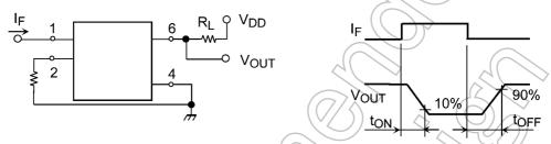
Fig. 11.1 Switching Time Test Circuit and Waveform
