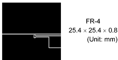
Fig. 5.1 Device Mounted on a Glass-Epoxy Board (a)
