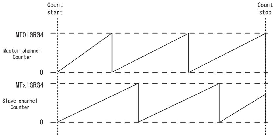
Figure 18-13 Synchronous start operation
