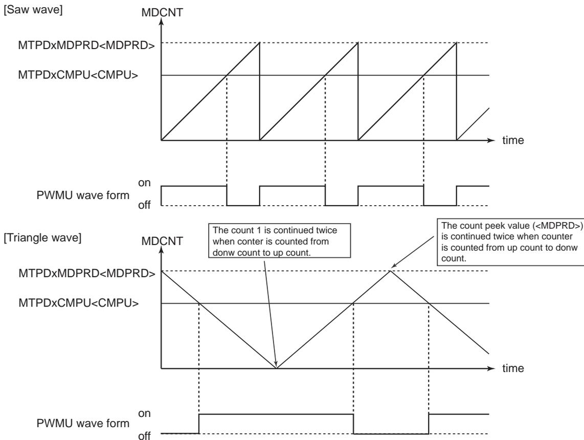
Figure 18-25 PWM waveform
