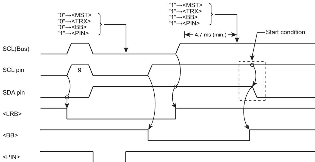
Figure 14-14 Timing Chart of Generating a Restart
