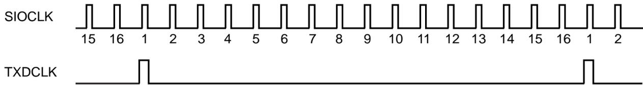
Figure 12-6 Generation of Transmission Clock in UART Mode
