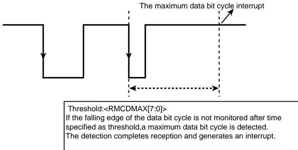
Figure 16-6 Completion by the maximum data bit cycle
