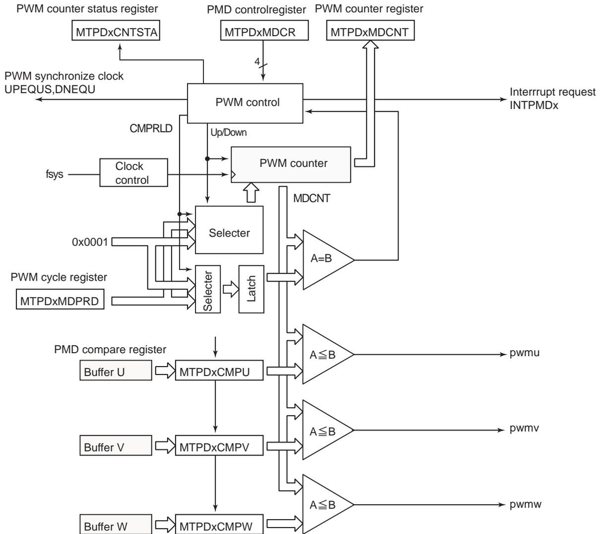
Figure 18-24 Schematic diagram of pulse width modulation circuit
