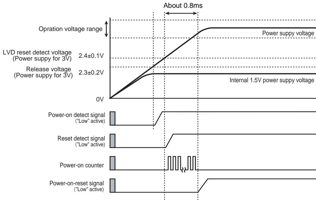
Figure 21-2 Power-on-reset operation timing
