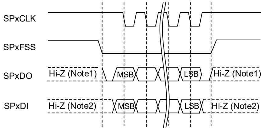
Figure 15-7 SPI frame format (single transfer, <SPO>="1" & <SPH>="0")
