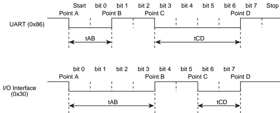
Figure 25-4 Serial Operation Mode Byte
