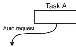
The DMA performs the task A. After completing the transfer, a transfer request is automatically generated and arbitration starts.
