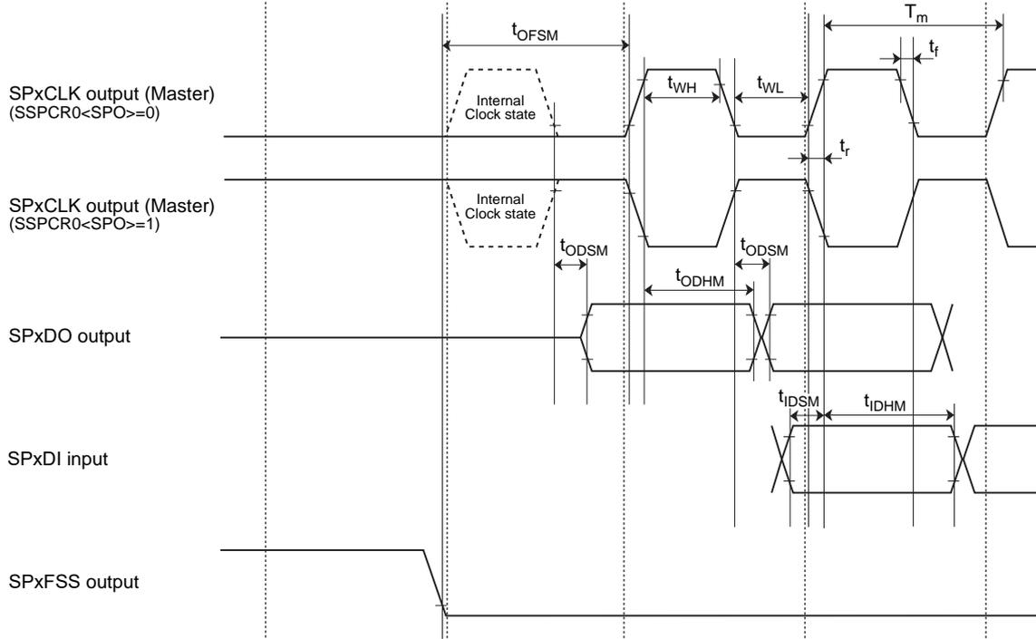
(2) Master SSPCR0<SPH>="1" (Data is latched on the second edge)
