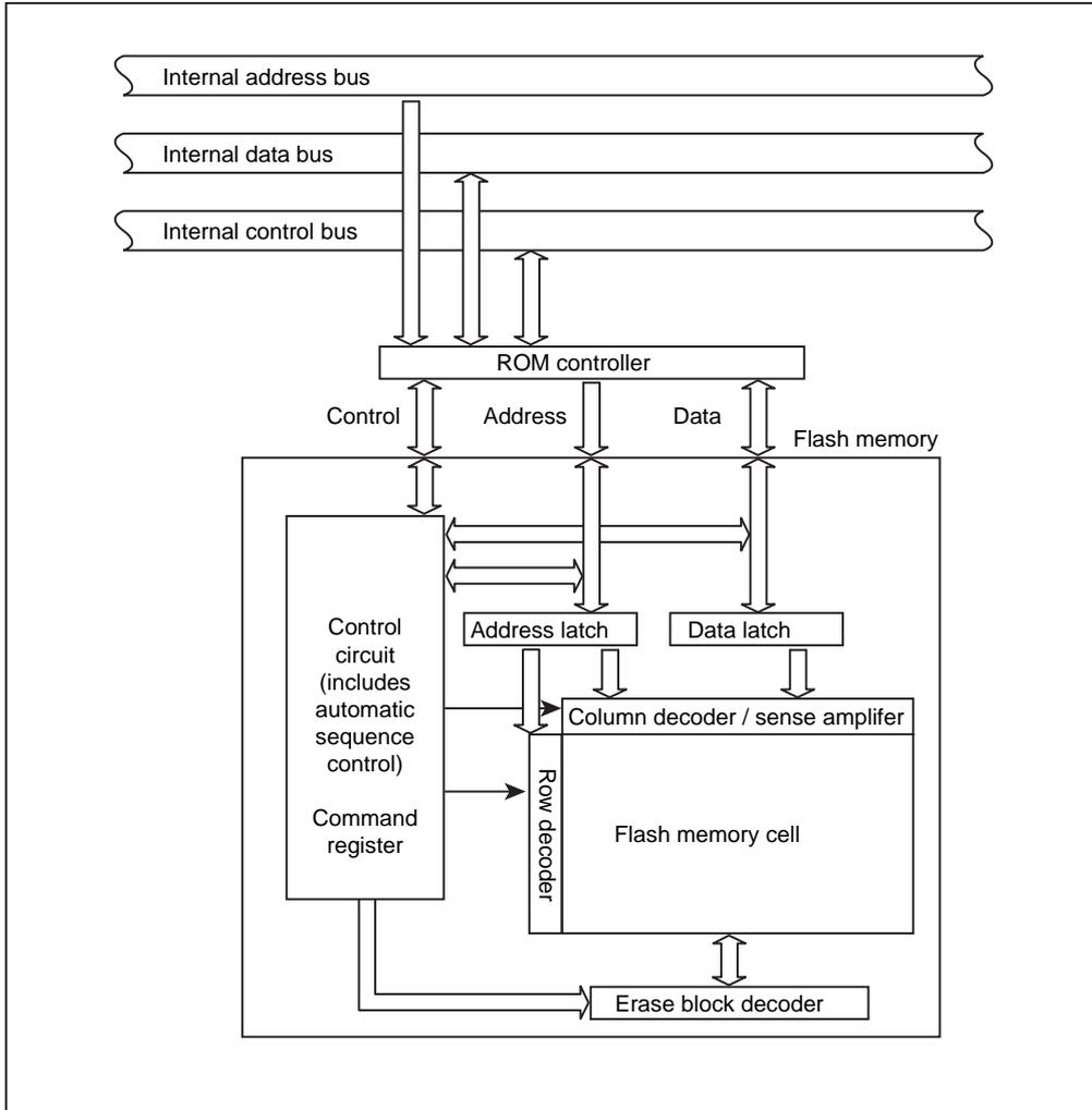
Figure 25-1 Block Diagram of the Flash Memory Section
