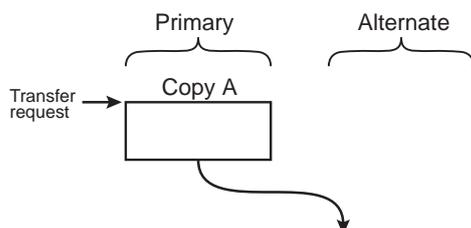
Receiving a transfer request, the DMA performs transfers for alternative data of the task A for four times.
