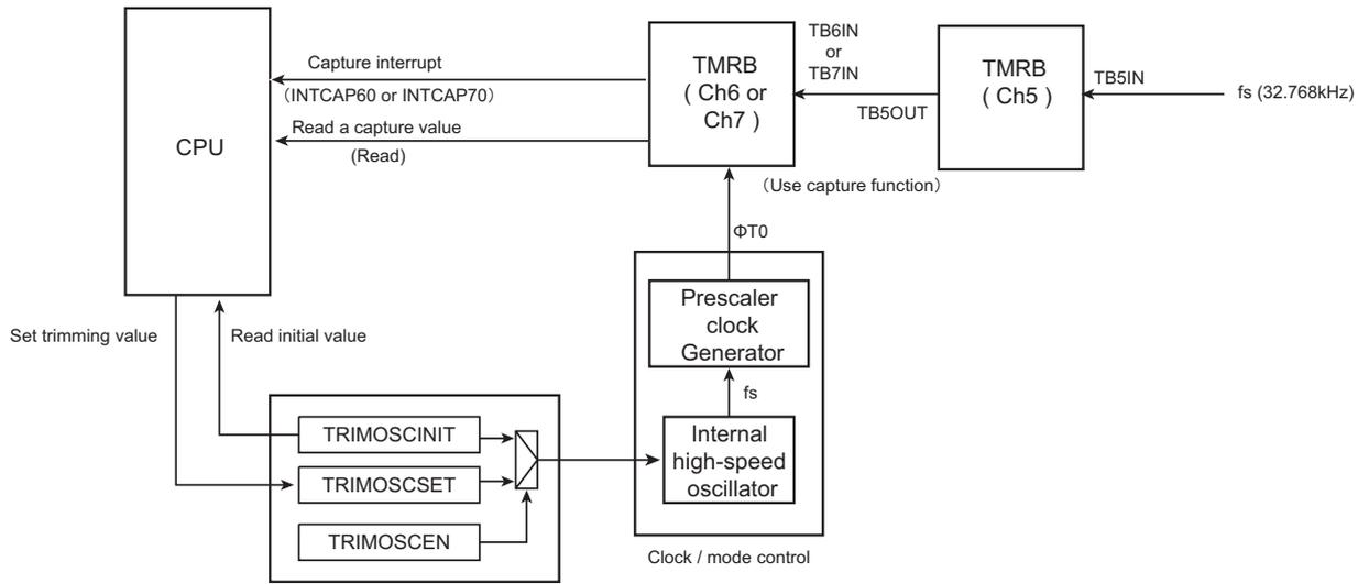
Figure 4-2 The way of input fs into TB5IN
