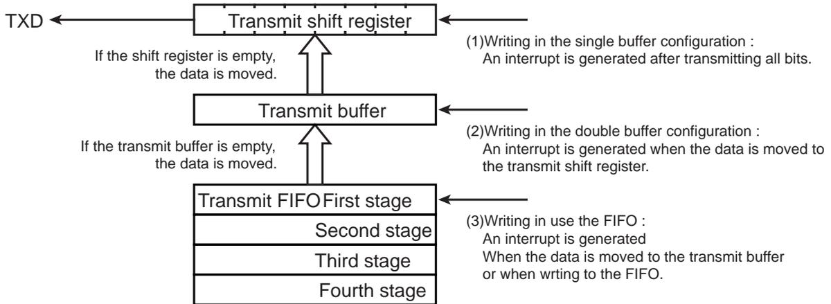
Figure 12-11 Transmit Buffer / FIFO Configuration Diagram
