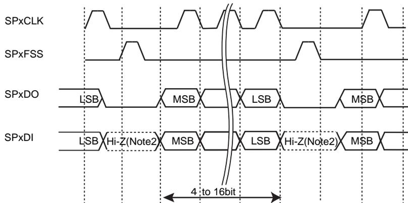
Figure 15-5 SPI frame format (continuous transfer, <SPO>="0" & <SPH>="0")
