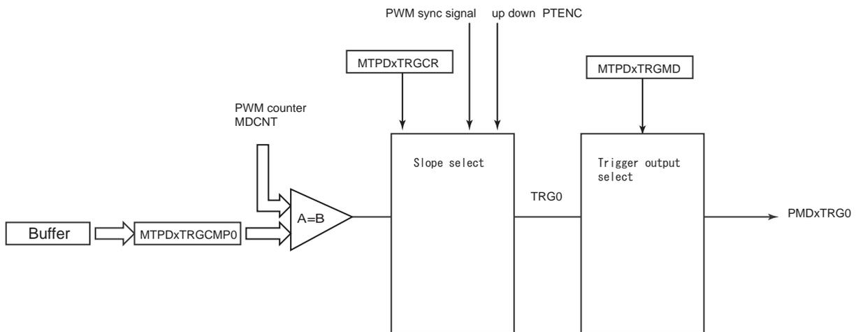
Figure 18-29 Schematic diagram of synchronous trigger generation circuit
