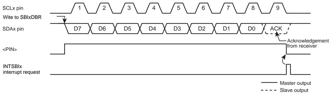
Figure 14-10 <BC[2:0]>= "000", <ACK>= "1" (Transmitter Mode)
