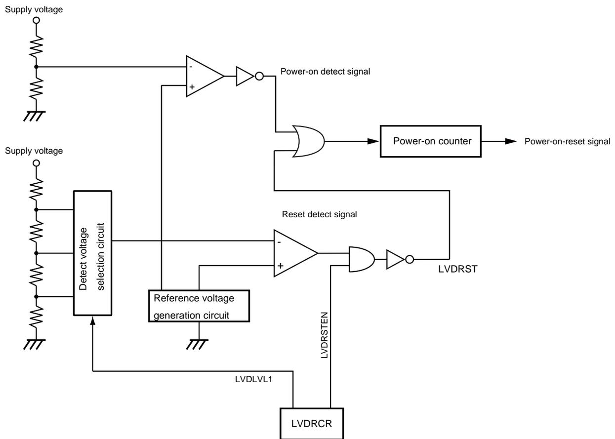
Figure 21-1 Power-on-reset circuit
