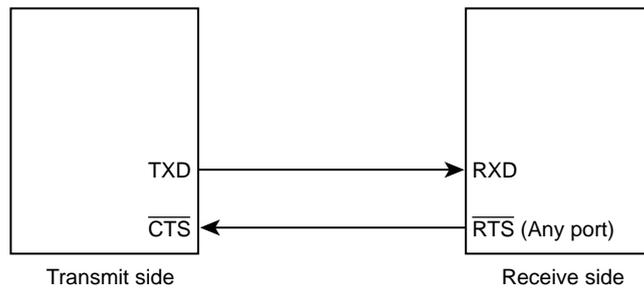
Figure 12-8 Handshake Function
