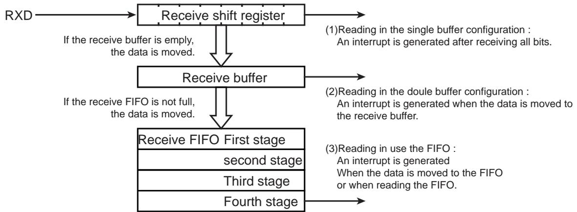
Figure 12-10 Receive Buffer / FIFO Configuration Diagram
