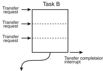
Receiving a transfer request, the DMA performs a transfer four times and performs arbitration.
