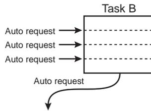
The DMA performs the task B. After completing the transfer, a transfer request is automatically generated and arbitration starts.
