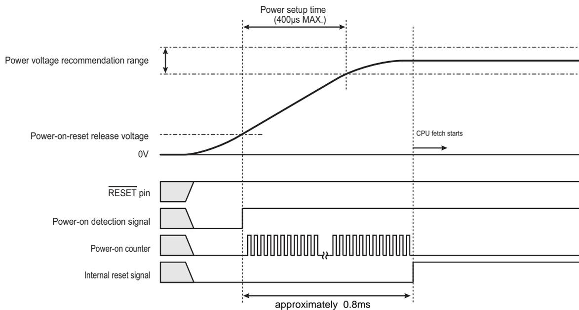
Figure 6-1 Reset Operation by Power-on Circuit
