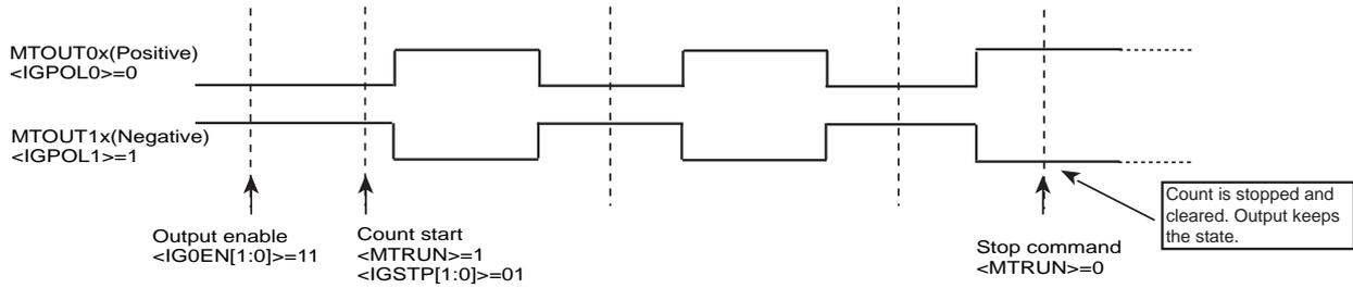
Figure 18-16 Counter stops with maintaining the output status
