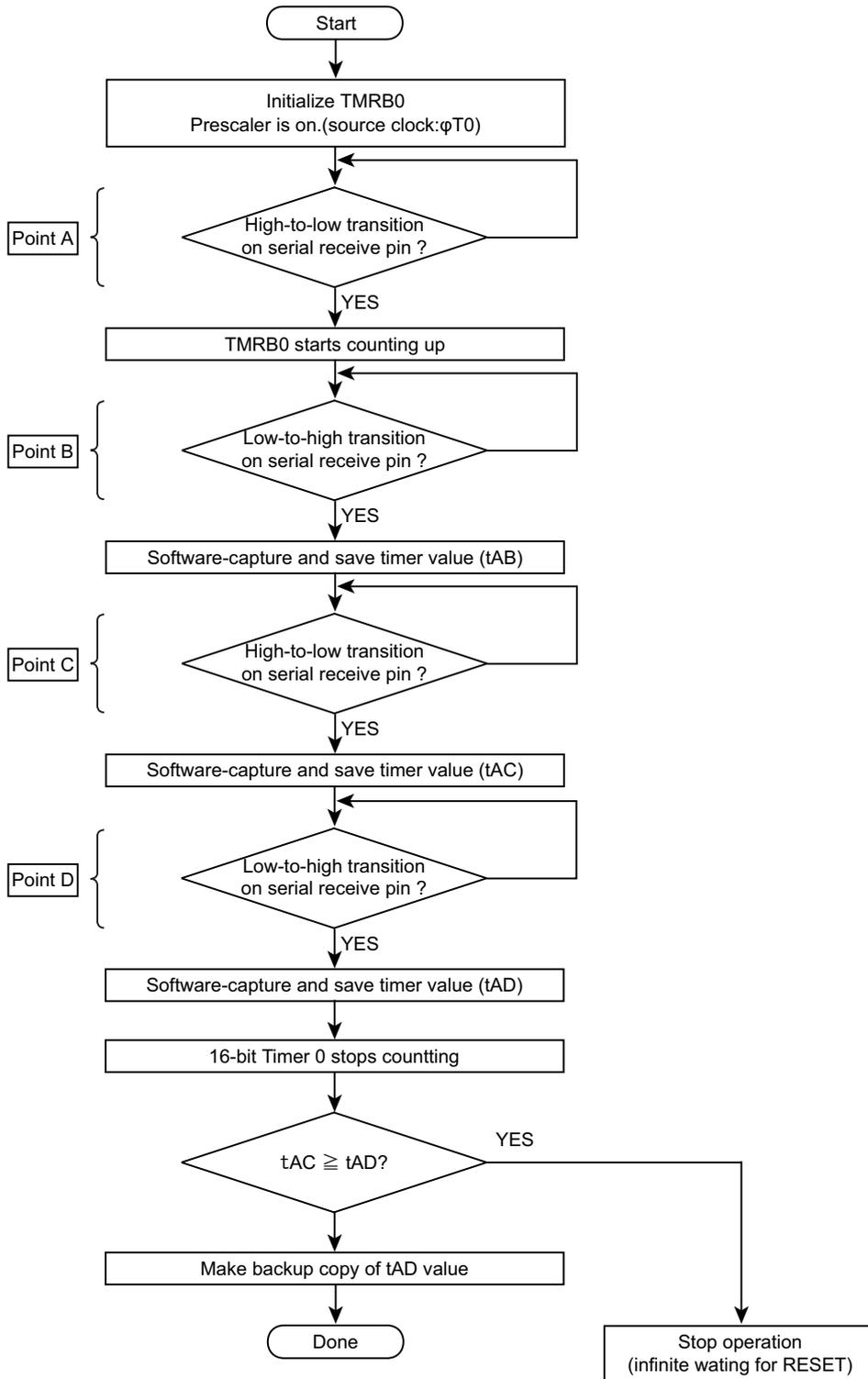
Figure 25-5 Serial Operation Mode Byte Reception Flowchart
