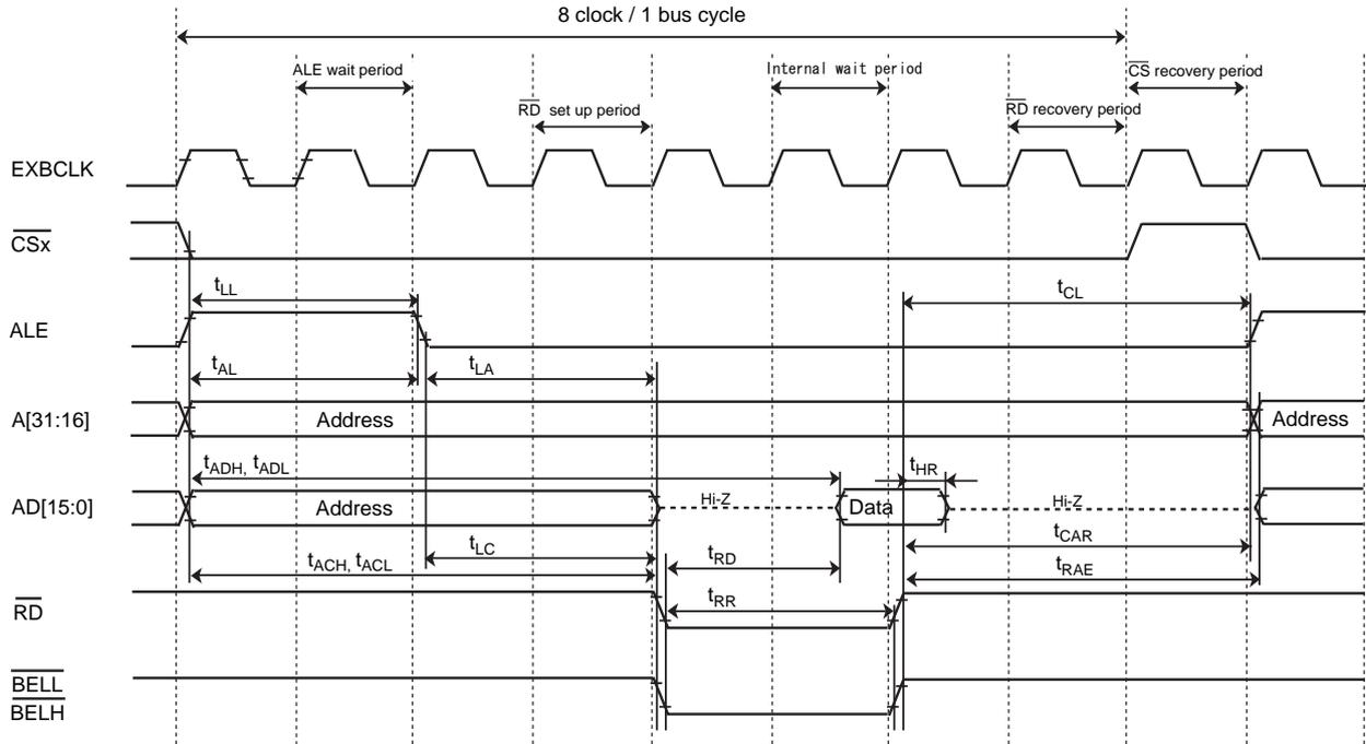
Read cycle timing (1 bus cycle per 9 clock)
