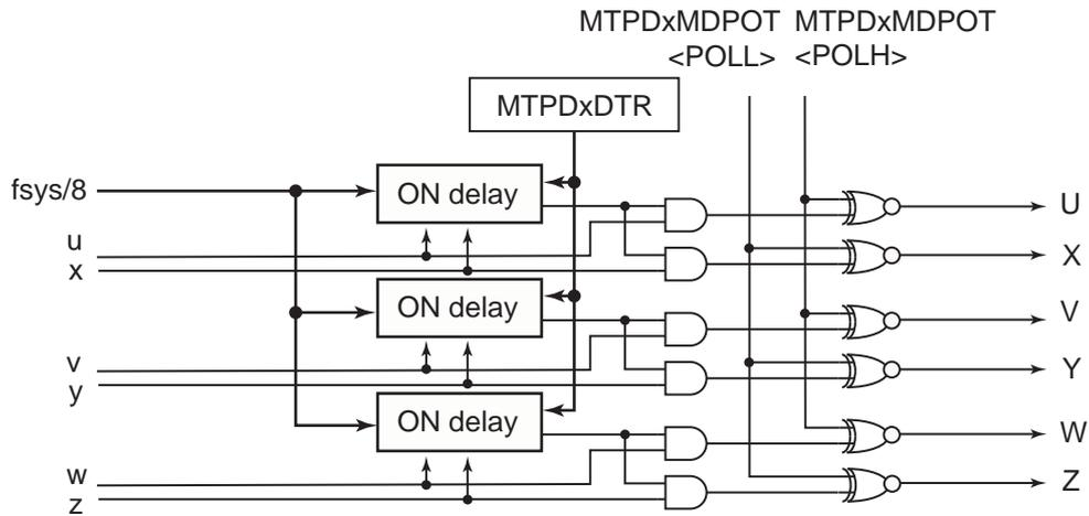
Figure 18-28 Schematic diagram of dead time circuit
