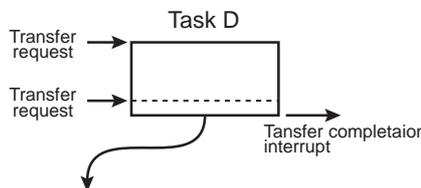
Receiving a transfer request, the DMA performs a transfer four times and performs arbitration.
