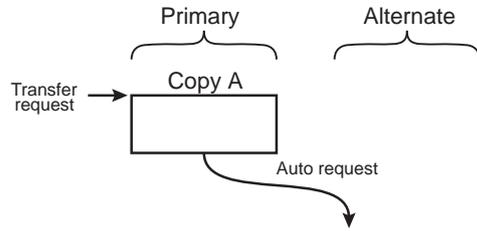
Receiving a transfer request, the DMA performs a transfer for alternative data of the task A for four times. After completing the transfer, a transfer request is automatically generated and arbitration starts.
