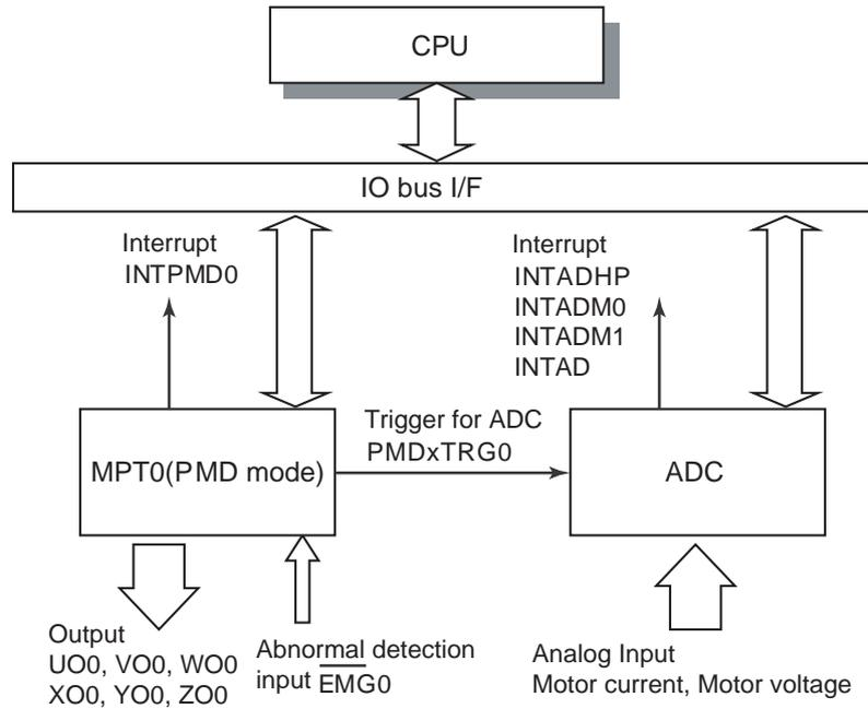
Figure 18-22 Block diagram of related with motor control
