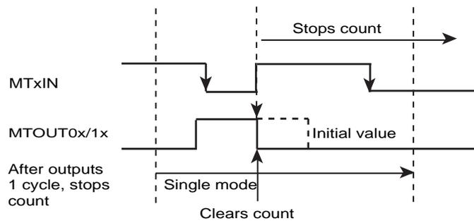
Figure 18-19 Trigger acceptance while cycles are stopping
