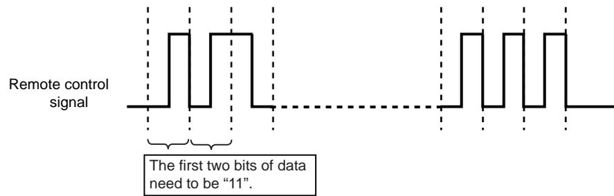
Figure 16-11 The waveform pattern in phase method
