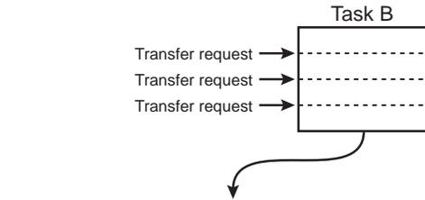
The DMA performs the task B. Since an arbitration occurs every 2<sup>R</sup> times of transfers, three times of transfer is required at least to complete the task B.
