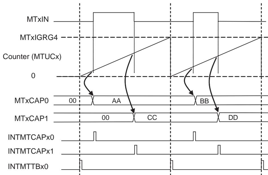
Figure 18-10 Capture operation
