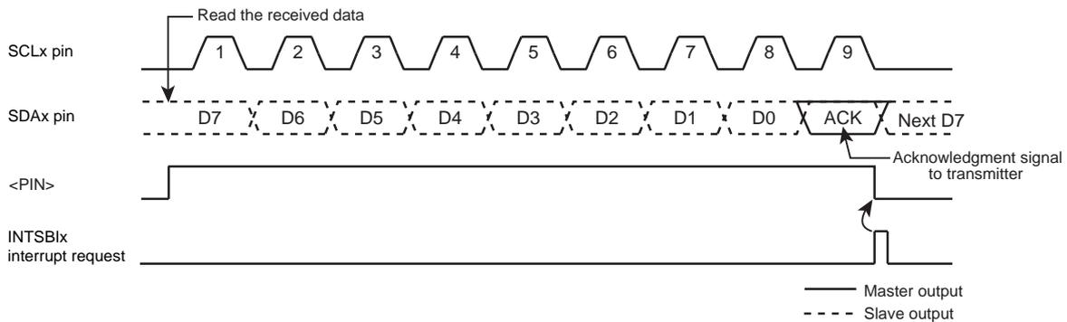
Figure 14-11 <BC[2:0]>= "000", <ACK>= "1" (Receiver Mode)
