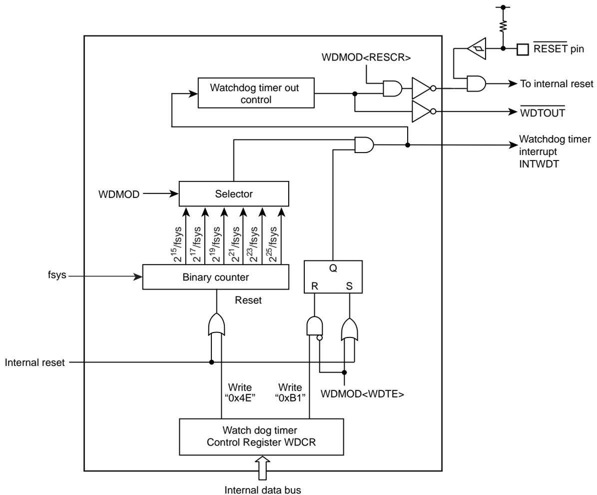
Figure 24-1 Block Diagram of the Watchdog Timer
