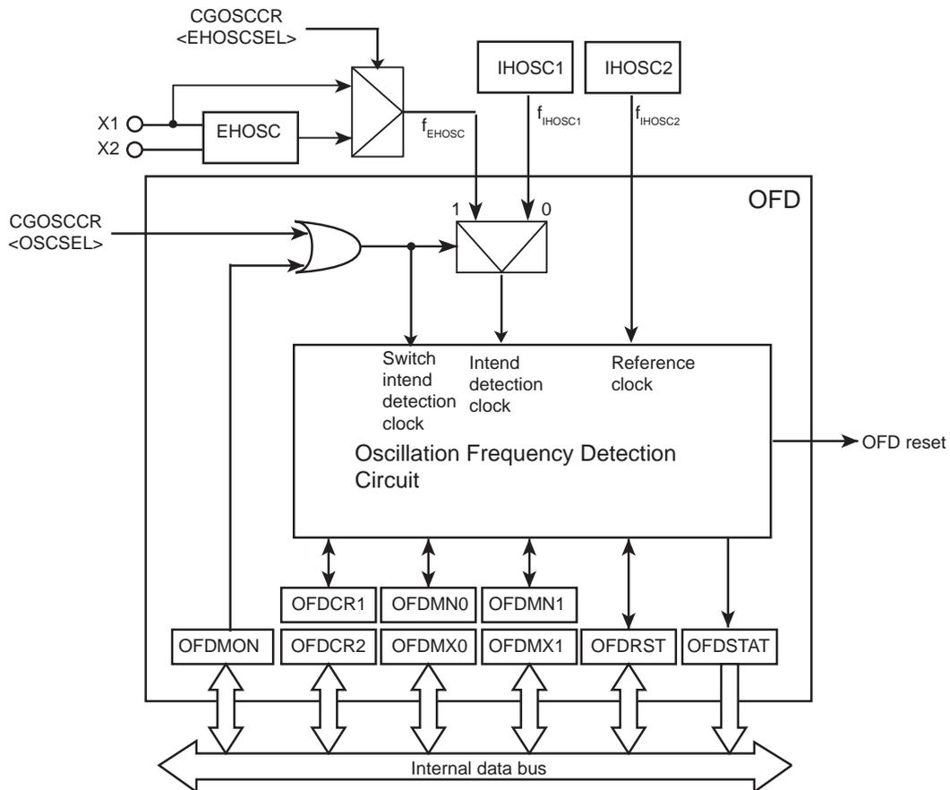
Figure 23-1 Oscillation Frequency Detector Block diagram
