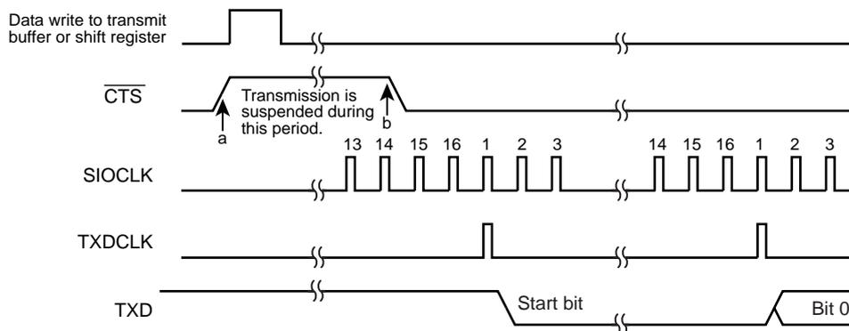
Figure 12-9  $\overline{CTS}$  Signal timing
