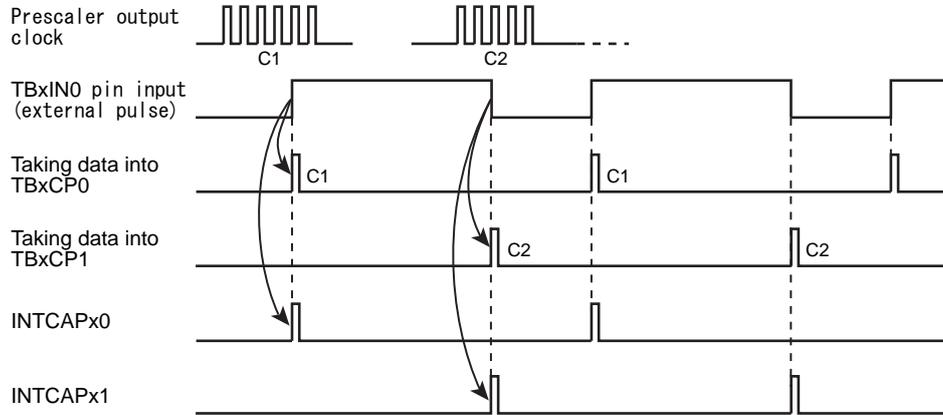
Figure 11-8 Pulse Width Measurement
