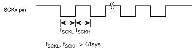
Figure 14-16 Maximum Transfer Frequency of External Clock Input
