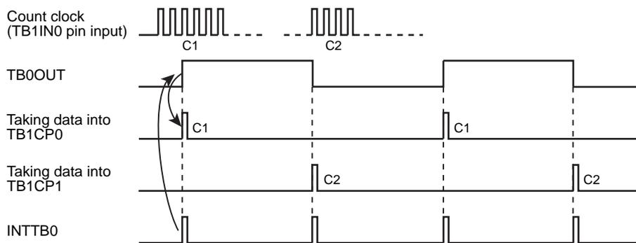
Figure 11-7 Frequency Measurement
