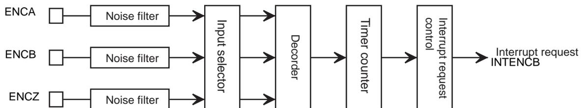
Figure 19-1 Block diagram of encoder input circuit
