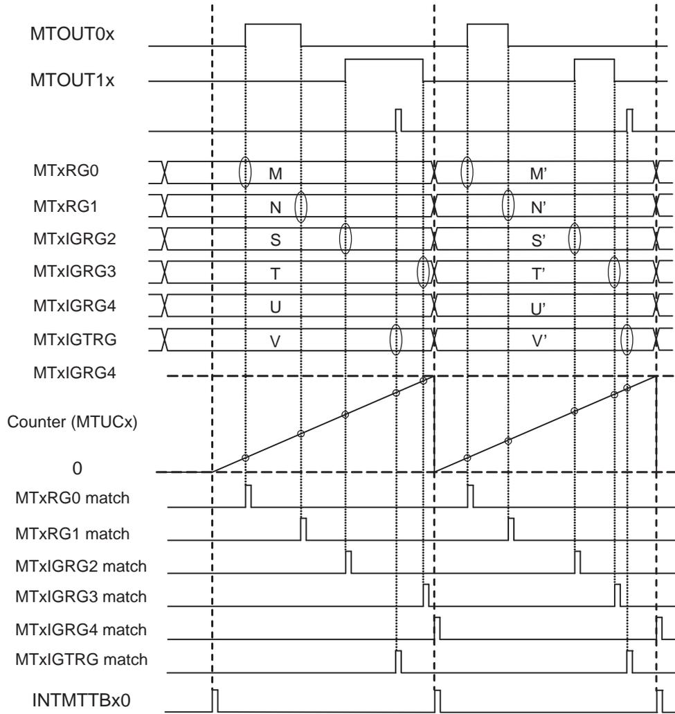
Figure 18-8 IGBT mode basic timing
