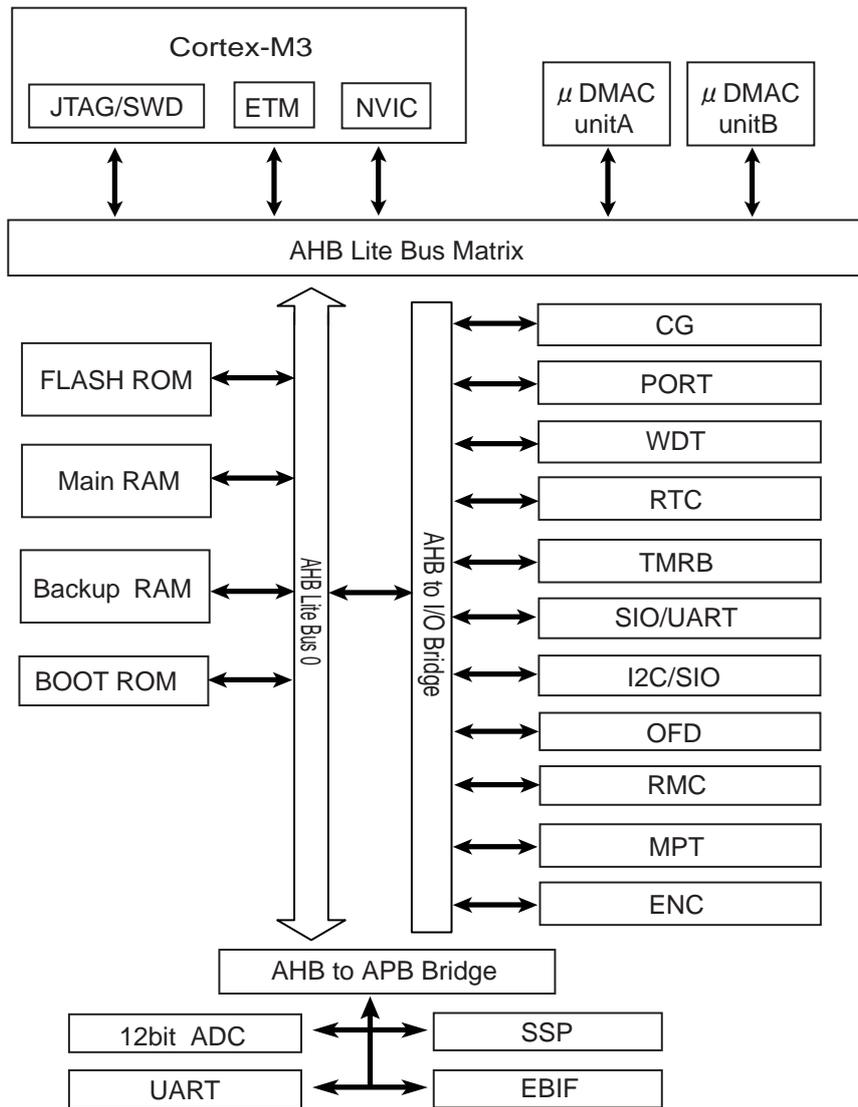
Figure 1-1 TMPM36BFYFG Block Diagram
