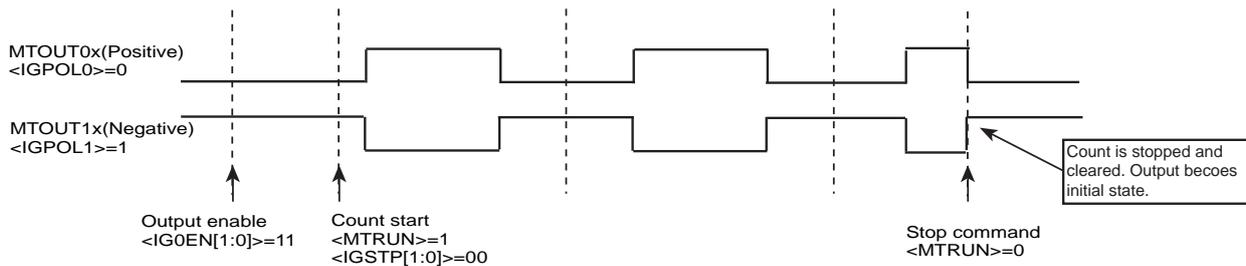
Figure 18-15 Counter stops with initial state output
