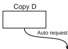
The DMA performs transfers for alternative data of the task D for four times. The DMA also sets "000" to `<cycle_ctrl>` of the primary data in order to set the next primary data invalid. A transfer request is automatically generated and arbitration starts.
