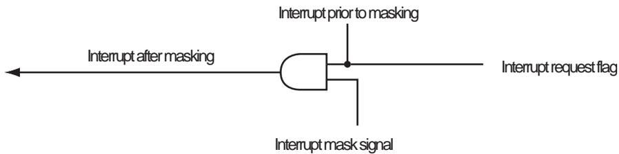
• The interrupt request flag state by the overrun error <OE> flag changes in real time and its state is not retained. And the <OE> flag is cleared by a read of receive FIFO.
