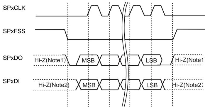
Figure 15-4 SPI frame format (single transfer, <SPO>="0" & <SPH>="0")
