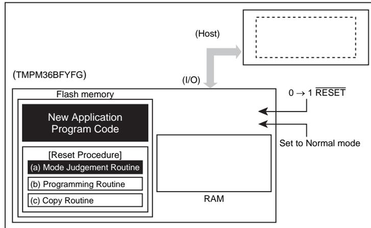
25.2.2.2 (1-B) Method 2: Transferring a Programming Routine from an External Host
