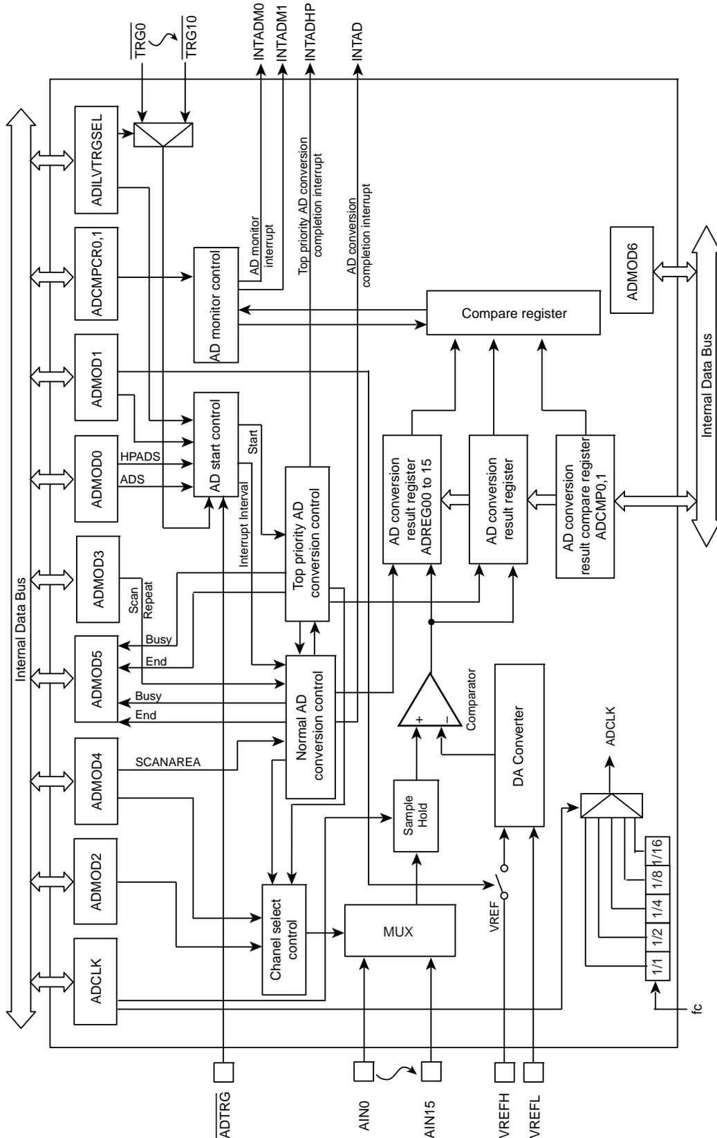
Figure 17-1 Block Diagram
