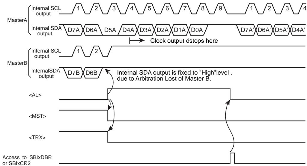
Figure 14-8 Example of Master B Lost Arbitration (D7A = D7B, D6A = D6B)
