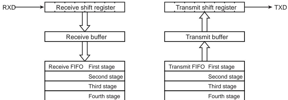
Figure 12-3 The Configuration of Buffer and FIFO
