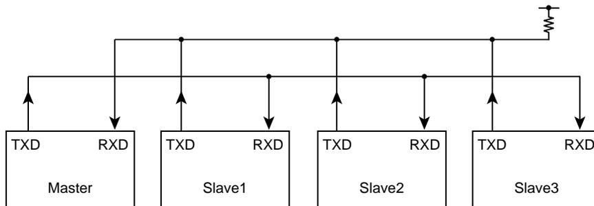
Figure 12-18 Serial Links to Use Wake-up Function
