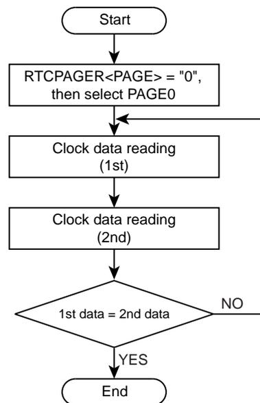
Figure 20-2 Flowchart of the clock data reading
