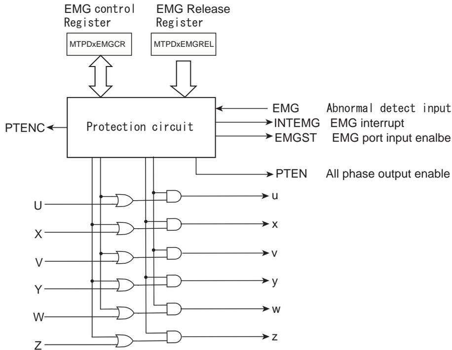
Figure 18-27 Schematic diagram of protection control circuit
