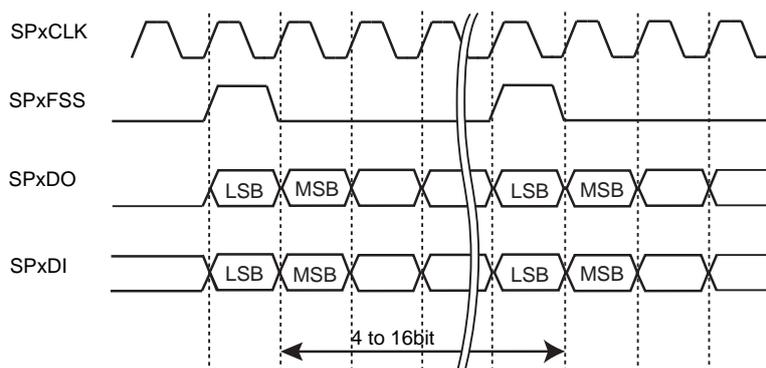
Figure 15-3 SSI frame format (transmission/reception during continuous transfer)
