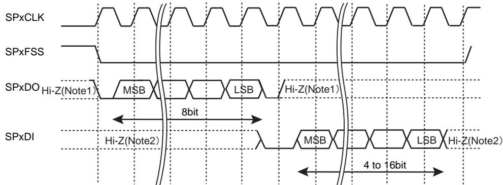
Figure 15-10 Microwire frame format (single transfer)
