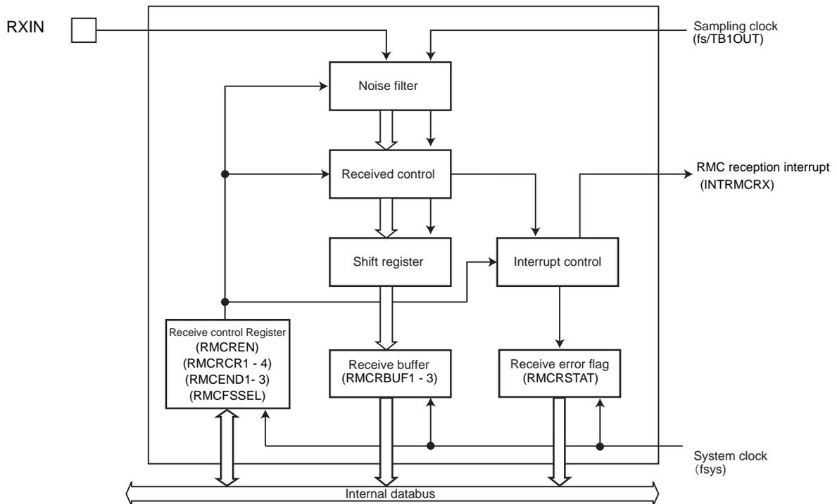
Figure 16-1 Block diagram of RMC
