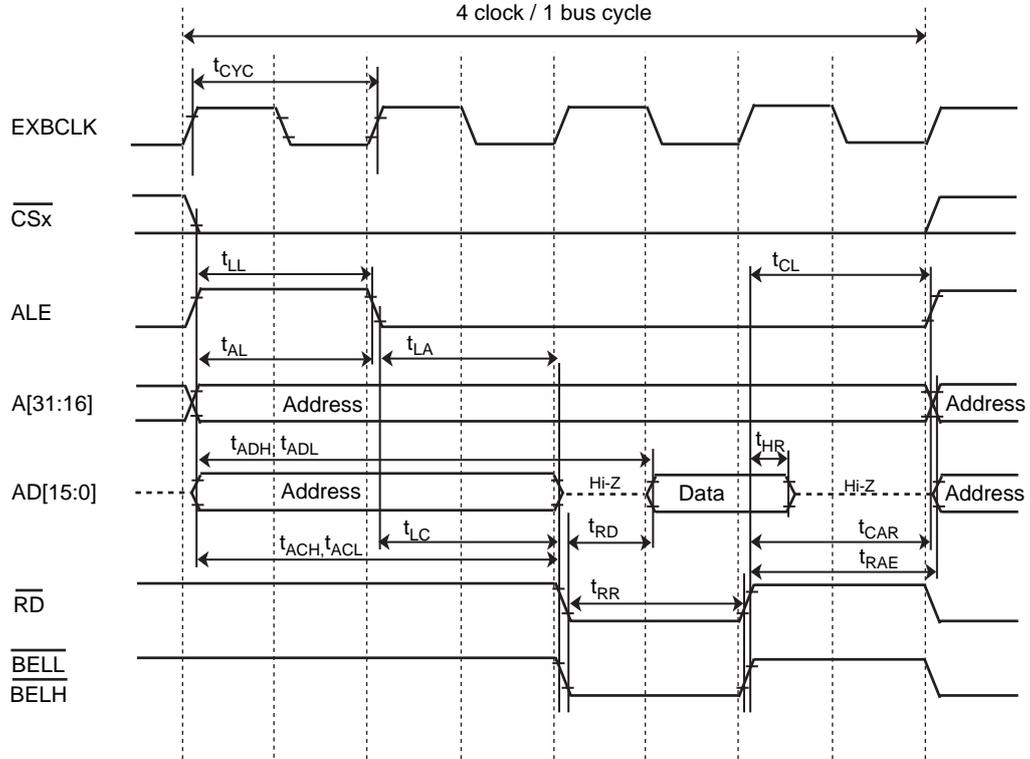
Read cycle timing (1 bus cycle per 8 clock)
