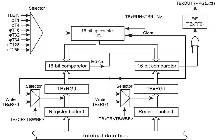
Figure 11-4 Block Diagram of 16-bit PPG Mode
