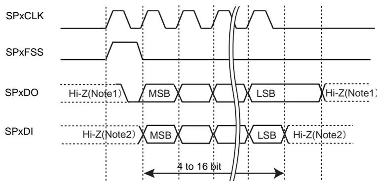
Figure 15-2 SSI frame format (transmission/reception during single transfer)
