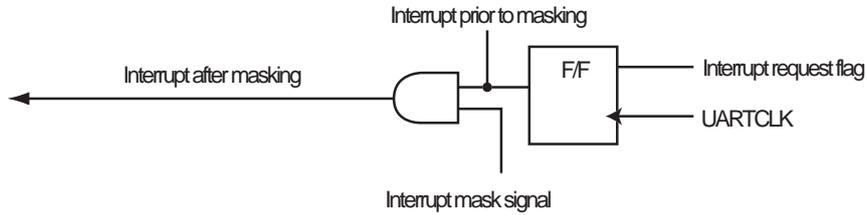
• The interrupt request flag state changes in real time and is retained in the F/F. Each flag can be cleared by a write to the corresponding bit in the interrupt clear register.
