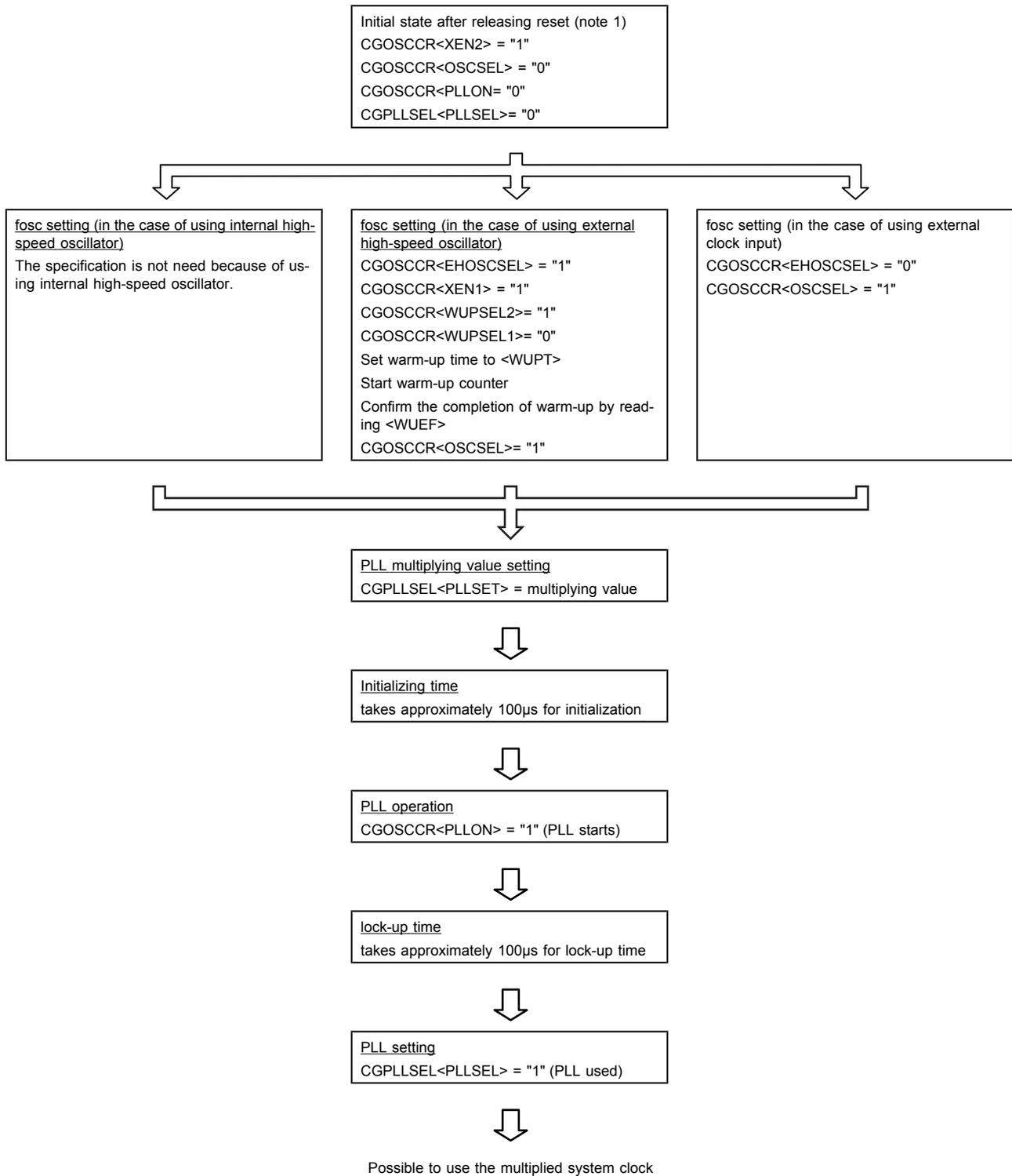
Note: Internal high-speed oscillator and voltage supply need to be stable.
