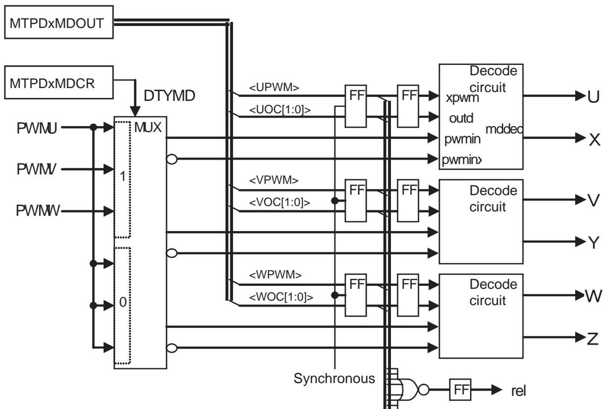
Figure 18-26 Schematic diagram of applying current control circuit
