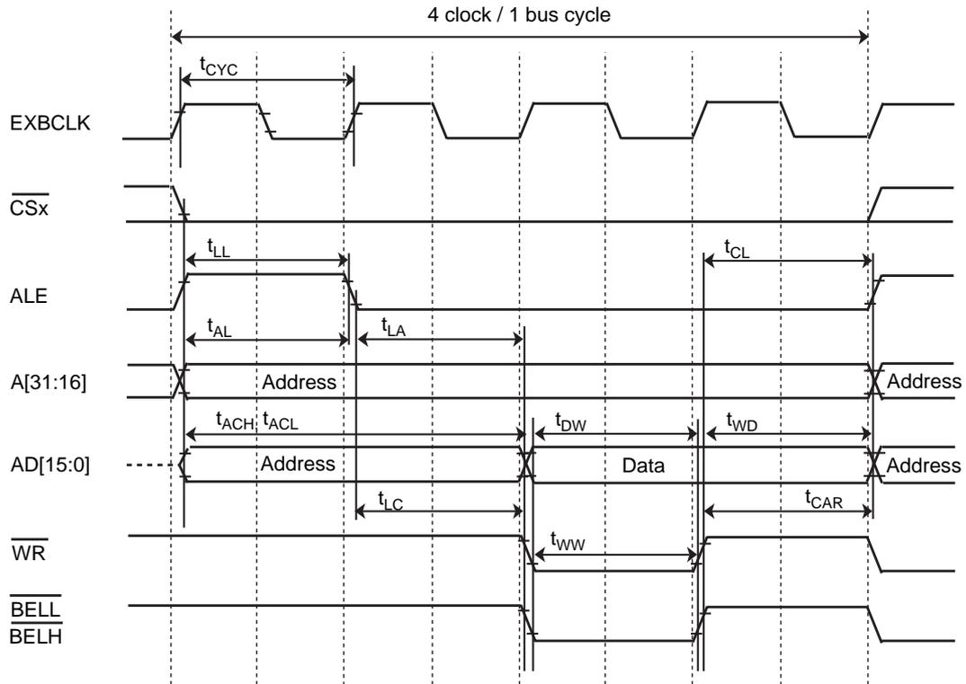
Write cycle timing (1 bus cycle per 8 clock)
