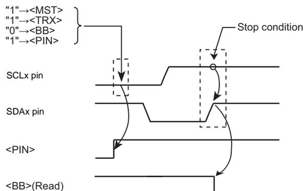
Figure 14-13 Generating the Stop Condition
