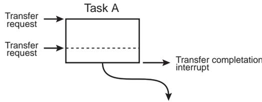
Receiving a transfer request, the DMA performs a transfer four times and performs arbitration.
