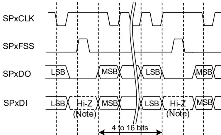
Figure 15-8 SPI frame format (continuous transfer, <SPO>="1" & <SPH>="0")
