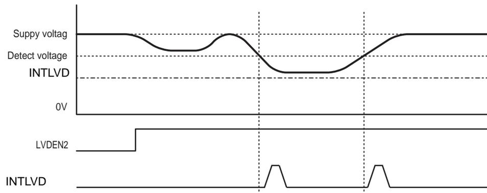
Figure 22-2 low voltage detection Timing
