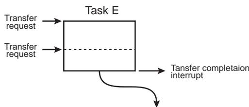
Receiving a transfer request, the DMA performs a transfer four times and performs arbitration.
