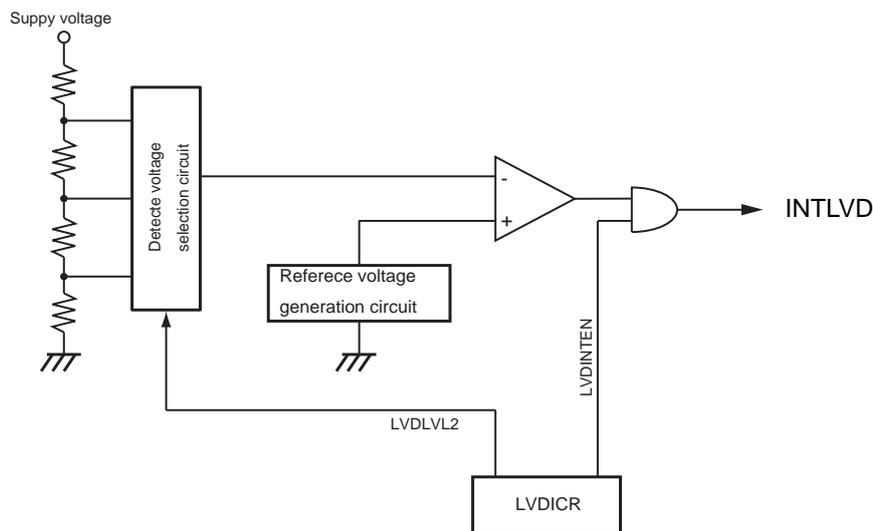
Figure 22-1 Block diagram of LVD (described only LVD interrupt circuit)
