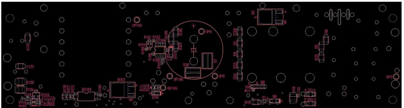
**Fig. 2.4 PCB Component Layout (Back Side)**
