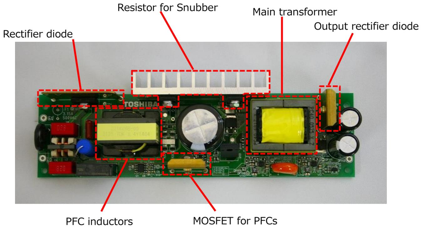
**Fig. 3.3 Parts and Area of High Heating Generation**
