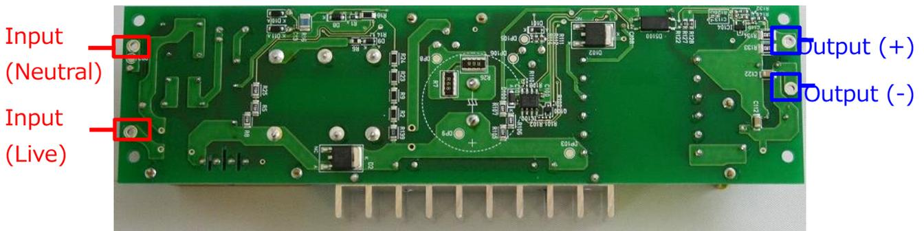
**Fig. 3.1 External connection terminals**
