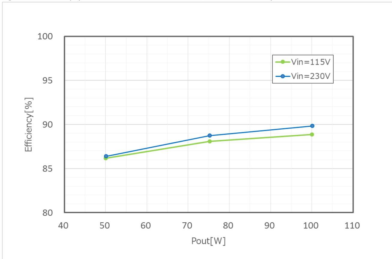
Fig. 4.1 Efficiency ( $I_{out} = 1.04 \text{ A}$ ,  $V_{inAC} = 115 \text{ V}$ ,  $V_{inAC} = 230 \text{ V}$ )
