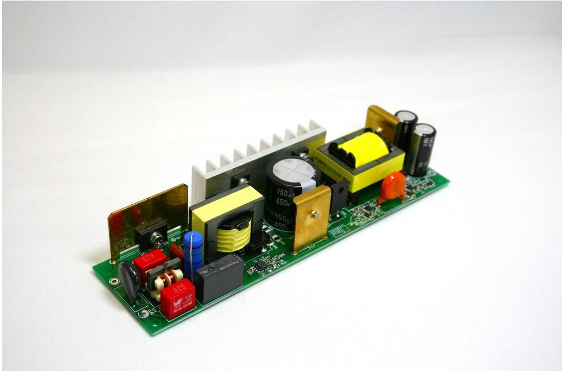
**Fig. 2.1 External View of 100 W Power Supply for LED Lighting**
