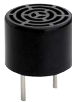
Fig. 2.3 Ultrasonic Transducer (C4016A1 made by Nippon Ceramic)
