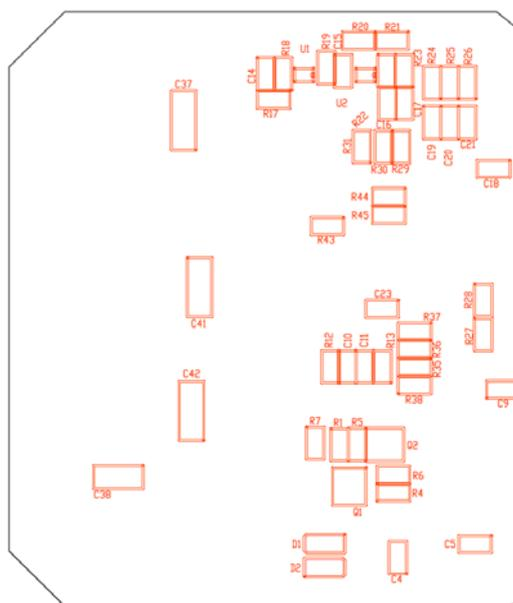
**Fig.4.4 Main Board Substrate Silk (Bottom side)**
