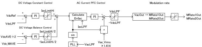
2. DC Voltage Constant Control and DC Voltage Balance Control
