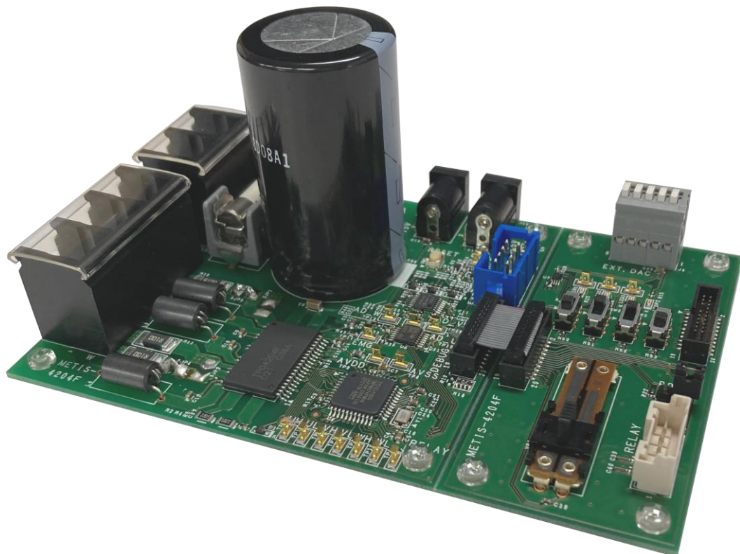
Fig. 2.3 DC 300 V Input BLDC Motor Sensorless Control Circuit External view of PCB (for RD179-3)
