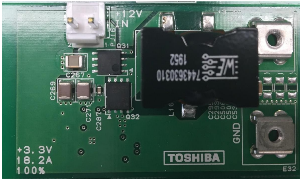
Fig. 3.1 External View of 3.3 V/18.2 A Output Power Supply Optimized for Efficiency at 100 % Load (Front Side)
