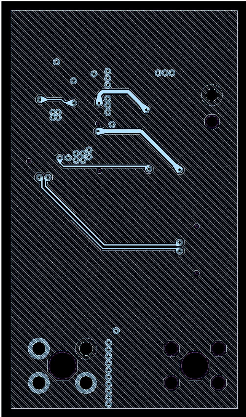
Fig. 3.7 PCB Pattern of 3.3 V/18.2 A Output Power Supply Optimized for Efficiency at 100 % Load (Layer 3)
