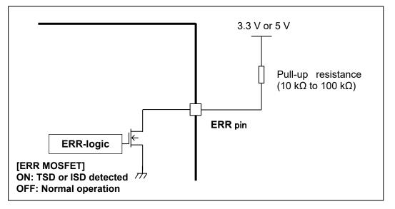
Figure 6.6 ERR pin equivalent circuit
