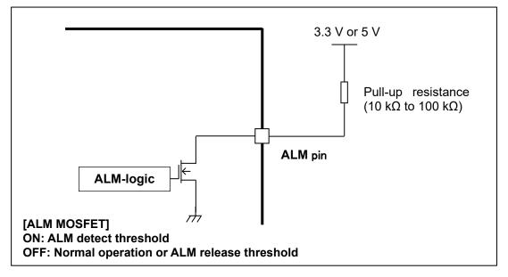
Figure 6.8 ALM pin equivalent circuit
