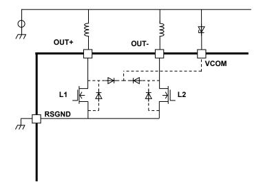
Figure 6.9 OFF TIME for PHASE switching equivalent circuit
