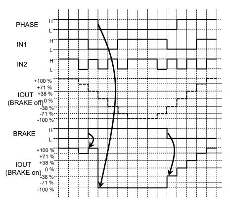
Figure 6.5 Relation between BRAKE mode and current setting
