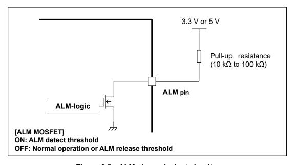
Figure 6.5 ALM pin equivalent circuit
