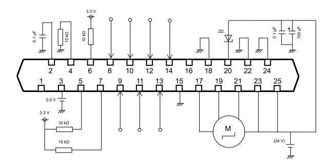
Figure 10.1 Application Circuit Example
