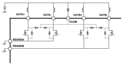
Figure 6.1 Break mode equivalent circuit
