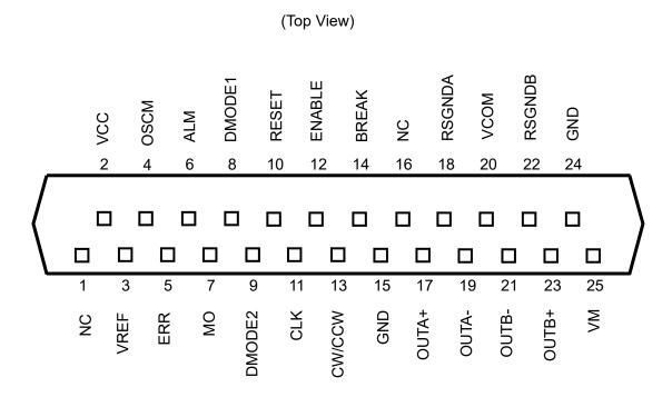
Figure 4.1 Pin Assignments (top view)
