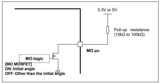
Figure 6.2 Monitor pin equivalent circuit
