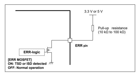
Figure 6.3 ERR pin equivalent circuit
