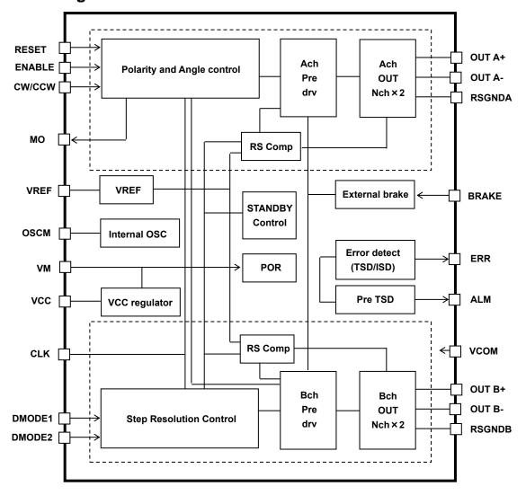
Figure 3.1 **Block Diagram**
