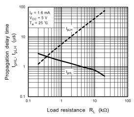
Fig. 12.2.16  $t_{pHL}$ , $t_{pLH}$  -  $R_L$
