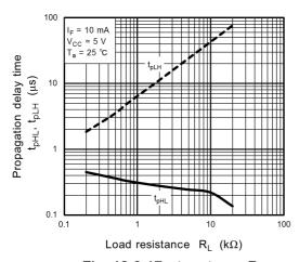
Fig. 12.2.17 t<sub>pHL</sub>,t<sub>pLH</sub> - R<sub>L</sub>
