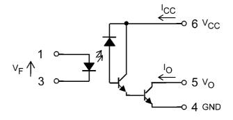
Note: A 0.1- $\mu F$  bypass capacitor must be connected between pin 6 and pin 4.
