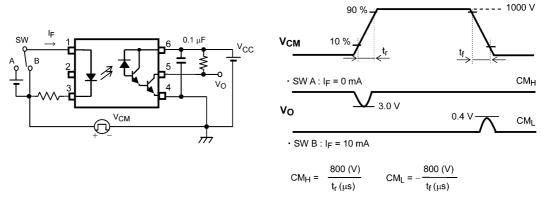
Fig. 12.1.2 Common-Mode Transient Immunity Test Circuit and Waveform
