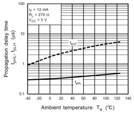
Fig. 12.2.14  $t_{pHL}$ , $t_{pLH}$  -  $T_a$
