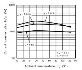
Fig. 12.2.9 I<sub>O</sub>/I<sub>F</sub> - T<sub>a</sub>
