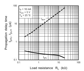
Fig. 12.2.18  $t_{pHL}$ , $t_{pLH}$  -  $R_L$
