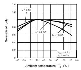
Fig. 12.2.10 I<sub>O</sub>/I<sub>F</sub> - T<sub>a</sub>
