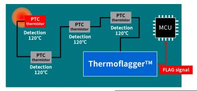
Abnormal heat generation is monitored by combining Thermoflagger<sup>TM</sup> and PTC thermistor located at the heat generating position.
