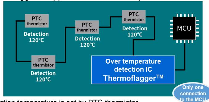
Detection temperature is set by PTC thermistor
