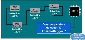
Detection temperature is set by PTC thermistor
