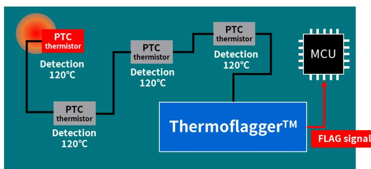
Abnormal heat generation is monitored by combining Thermoflagger™ and PTC thermistor located at the heat generating position.
