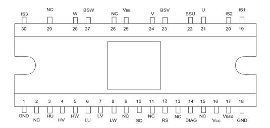
Figure 5.1 Pin Assignments
