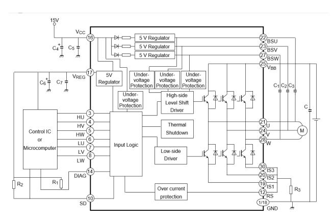
Figure 12.1 Application Circuit Example
