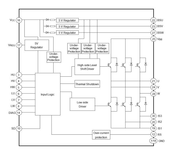
Figure 4.1 Block Diagram
