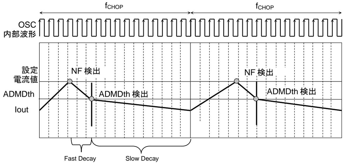
図 7.13 ADMD (Advanced Dynamic Mixed Decay)電流波形
