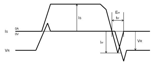
Fig. 7.6 Timing Chart(Diode part)
