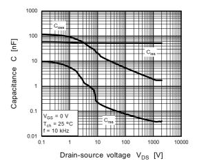
Fig. 8.6 C<sub>iss</sub>, C<sub>oss</sub>, C<sub>rss</sub> - V<sub>DS</sub>
