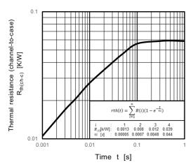
Fig. 8.13 R<sub>th(ch-c)</sub> - t (Guaranteed Maximum)
