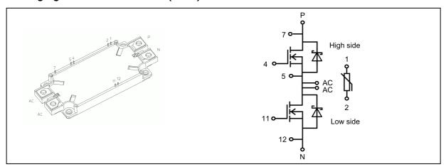
Note: P and N terminal should use one screw to fasten in each and AC terminal should use two screw to fasten. When the thermistor is not used, pin 1 and 2 should be electrically connected to pin 12.
