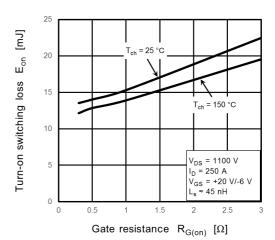
Fig. 8.10 E<sub>on</sub> -R<sub>G(on)</sub>
