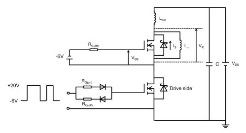
Fig. 7.5 Inductive Load Reverse Recovery Test Circuit(Low side Switching)
