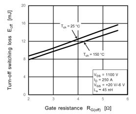
Fig. 8.11  $E_{off} - R_{G(off)}$
