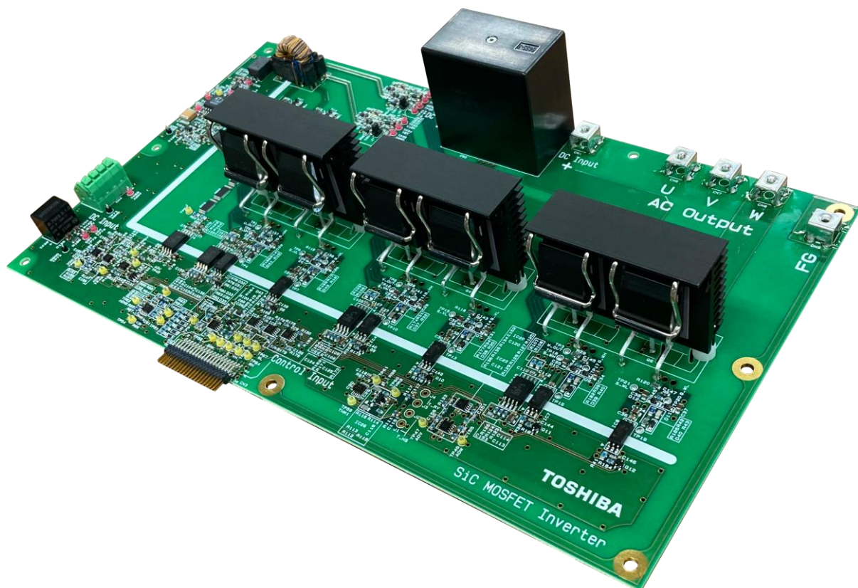
Fig. 2.5 3-Phase Inverter Using SiC MOSFET (Inverter Board with TW045N120C) Side View
