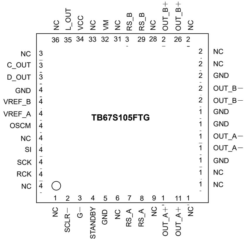
Figure3 Pin assignment
