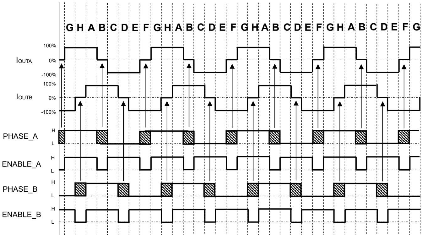
Figure 21.2.2 Half step resolution sequence timing chart
