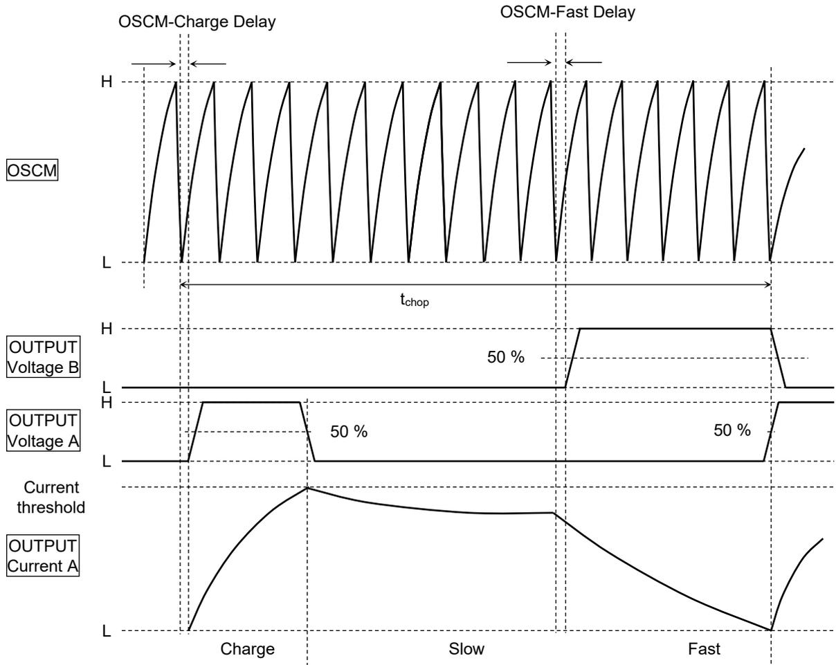
**Figure20.1 OSCM-Charge DELAY**
