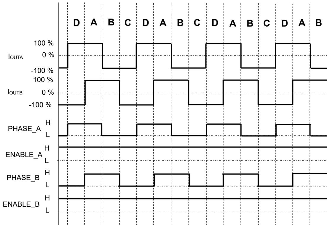
Figure 21.1.2 Full step resolution sequence timing chart
