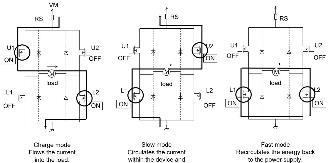
**Figure16 Motor output MOSFET operation mode**
