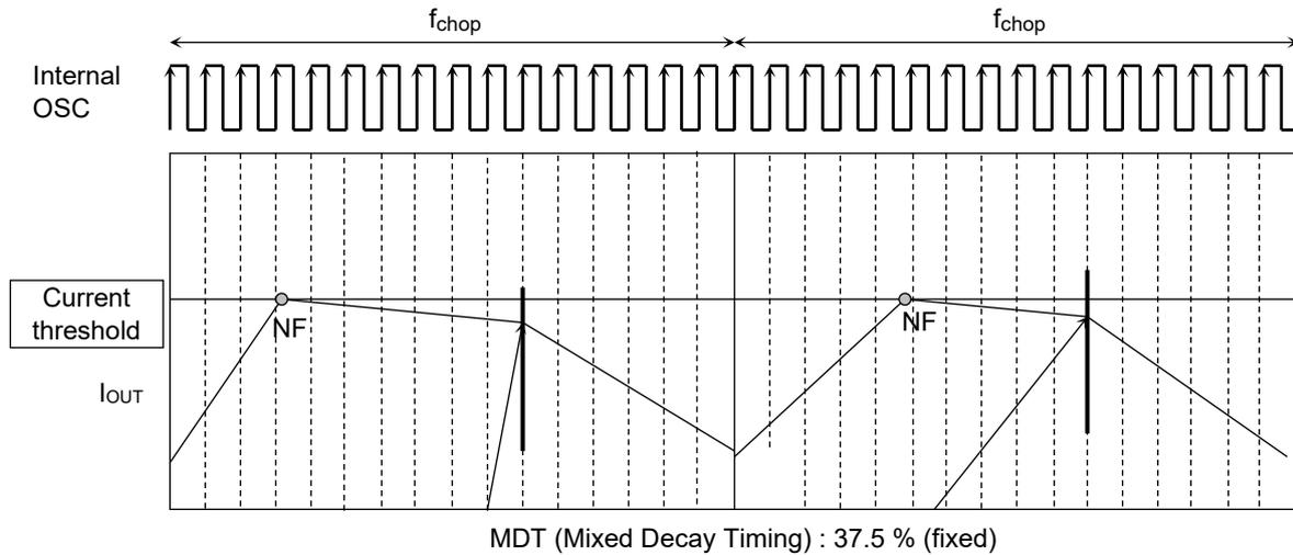
Figure 14.1 Mixed Decay Mode waveform (Current waveform)
