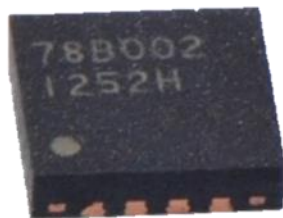
WQFN16 Package (3 x 3 x 0.75 mm)
