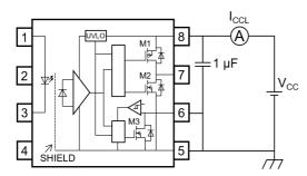
Fig. 13.1.7 I<sub>CCL</sub> Test Circuit
