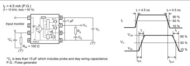
Fig. 13.1.8 Switching Time Test Circuit and Waveform
