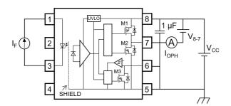
Fig. 13.1.1 I<sub>OPH</sub> Test Circuit
