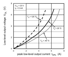
Fig. 13.2.9 V<sub>OL</sub> - I<sub>OPL</sub>
