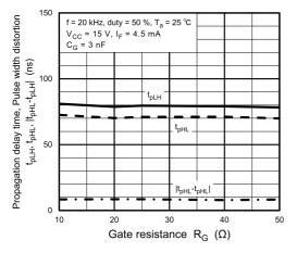
Fig. 13.2.21  $t_{pHL}$ ,  $t_{pLH}$ ,  $|t_{pHL}-t_{pLH}| - R_g$
