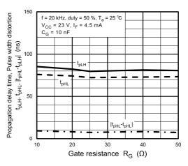
Fig. 13.2.22  $t_{pHL}$ ,  $t_{pLH}$ ,  $|t_{pHL}-t_{pLH}| - R_g$
