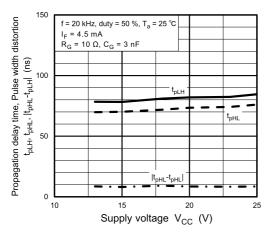
Fig. 13.2.19  $t_{pHL}$ ,  $t_{pLH}$ ,  $|t_{pHL}-t_{pLH}| - V_{CC}$
