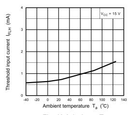
Fig. 13.2.4 I<sub>FLH</sub> - T<sub>a</sub>
