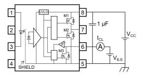
Fig. 13.1.5 I<sub>CLAMP</sub> Test Circuit
