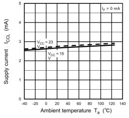
Fig. 13.2.5 I<sub>CCL</sub> - T<sub>a</sub>
