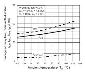
Fig. 13.2.15  $t_{pHL}$ ,  $t_{pLH}$ ,  $|t_{pHL}-t_{pLH}|$  -  $T_a$
