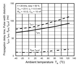
Fig. 13.2.16  $t_{pHL}$ ,  $t_{pLH}$ ,  $|t_{pHL}-t_{pLH}|$  -  $T_a$
