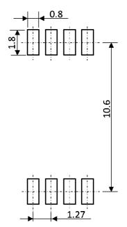
Fig. 15.2 Lead forming option (LF4)
