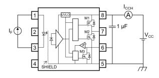
Fig. 13.1.6 I<sub>CCH</sub> Test Circuit
