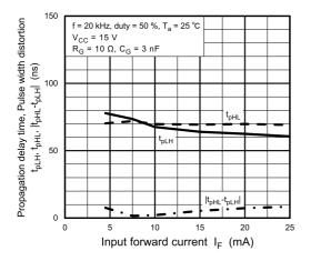
Fig. 13.2.17  $t_{pHL}$ ,  $t_{pLH}$ ,  $|t_{pHL}-t_{pLH}| - I_F$
