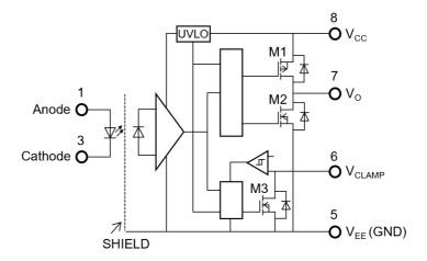
Note: A 1- $\mu$ F bypass capacitor must be connected between pin 8 and pin 5.
