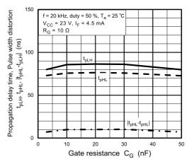
Fig. 13.2.24  $t_{pHL}$ ,  $t_{pLH}$ ,  $|t_{pHL}-t_{pLH}|$  -  $C_g$
