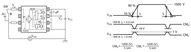
Fig. 13.1.9 Common-Mode Transient Immunity Test Circuit and Waveform
