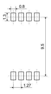
Fig. 15.1 Lead forming option (standard)
