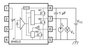
Fig. 13.1.4 V<sub>OL</sub> Test Circuit
