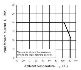
Fig. 13.2.2 I<sub>F</sub> - T<sub>a</sub>
