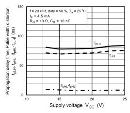
Fig. 13.2.20  $t_{pHL}$ ,  $t_{pLH}$ ,  $|t_{pHL}-t_{pLH}| - V_{CC}$
