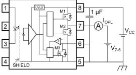
Fig. 13.1.2 I<sub>OPL</sub> Test Circuit
