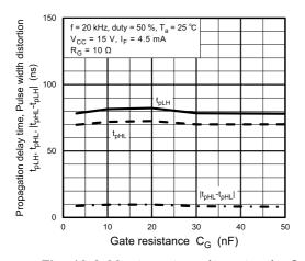
Fig. 13.2.23  $t_{pHL}$ ,  $t_{pLH}$ ,  $|t_{pHL}-t_{pLH}|$  -  $C_g$
