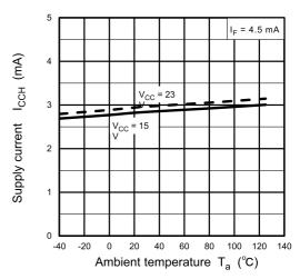
Fig. 13.2.6 I<sub>CCH</sub> - T<sub>a</sub>
