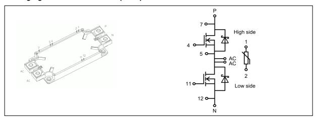
Note: P and N terminal should use one screw to fasten in each and AC terminal should use two screws to fasten. When the thermistor is not used, pin 1 and pin 2 should be electrically connected to pin 12.
