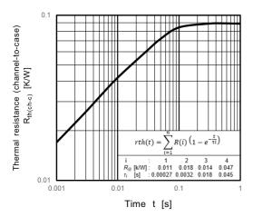
Fig. 8.13 R<sub>th(ch-c)</sub> - t (Guaranteed Maximum)
