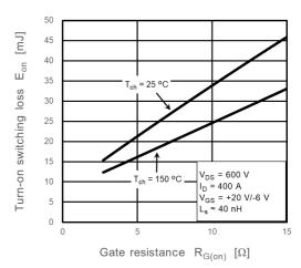
Fig. 8.10 E<sub>on</sub> -R<sub>G(on)</sub>
