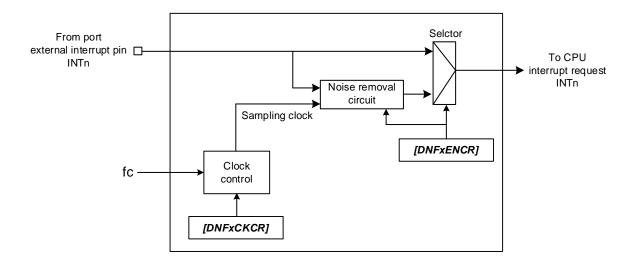
Figure 2.1 Digital Noise Filter Circuit Block Diagram
