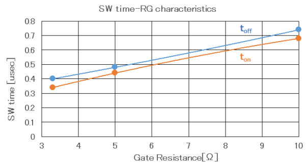
Fig. 4.13 Switching Time Characteristics
