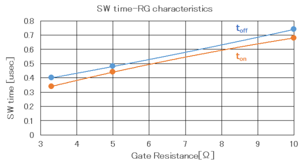
Fig. 4.13 Switching Time Characteristics
