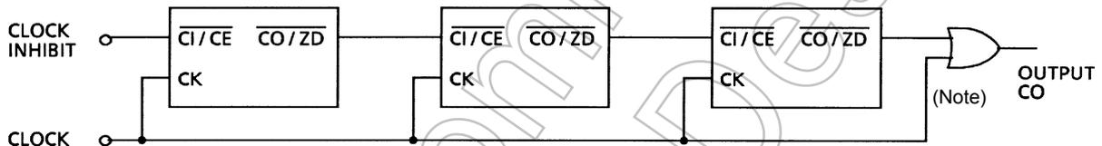
Note: At synchronous cascade connection, huzzerd occurs at CO output after its second stage when digit place changes, due to delay arrival. Therefore, take gate form TC74HC32A or the like, not form CO output at the rear stage directly.
