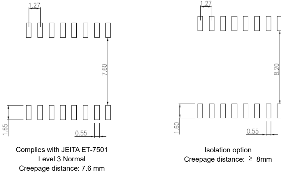
Figure 13.2 Land Pattern Dimensions for Reference only
