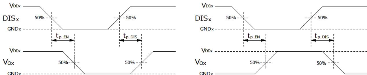
**Figure 8.2 Disable Propagation Delay Time Test Waveform Diagram**
