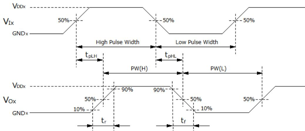
**Figure12.4 Switching Waveforms**
