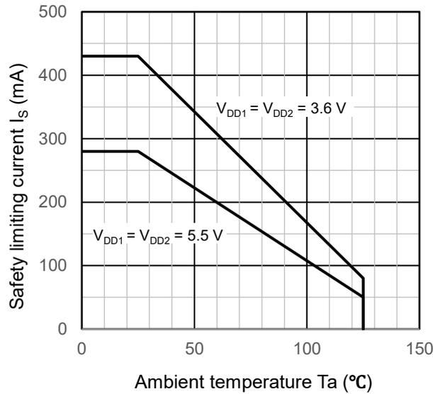
**Figure 9.1 Thermal derating curve for safety limiting current**
